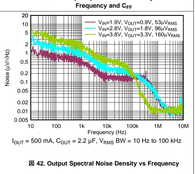
42. Output Spectral Noise Density vs Frequency
