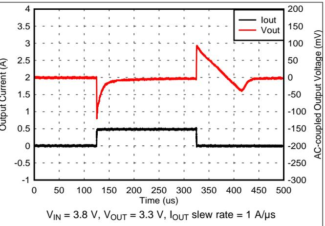
Figure 26. 3.3-V, 1-mA to 500-mA Load Transient
