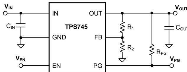
Figure 44. Adjustable Operation
