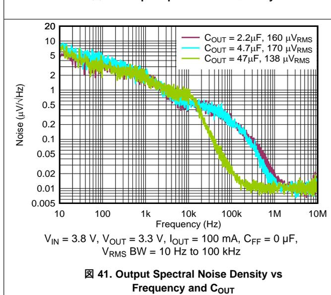
41. Output Spectral Noise Density vs Frequency and  $C_{OUT}$
