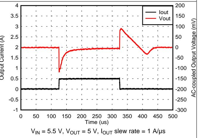
Figure 28. 5-V, 1-mA to 500-mA Load Transient
