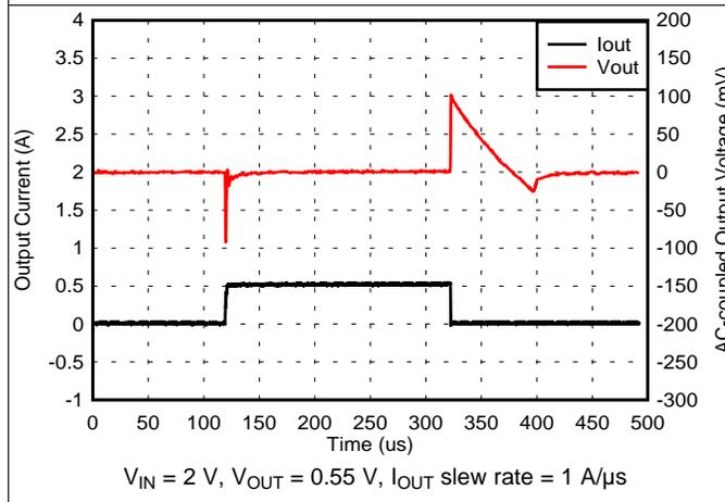
Figure 27. 0.55-V, 1-mA to 500-mA Load Transient
