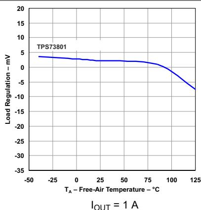
図 5-19. Load Regulation vs Temperature
