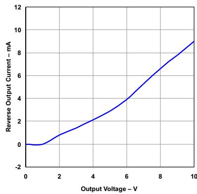
図 5-16. Reverse Output Current vs Output Voltage
