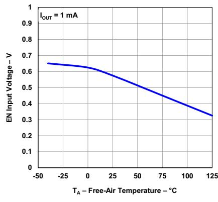
図 5-12. EN Threshold (On to Off) vs Temperature
