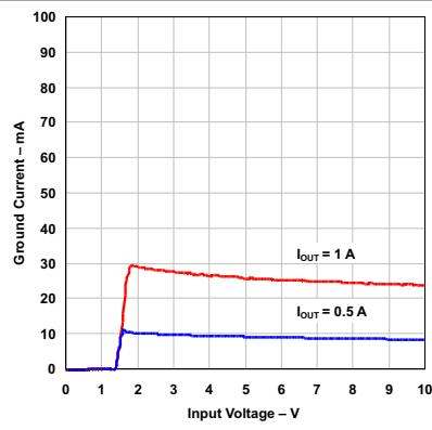
図 5-6. Ground Current vs Input Voltage
