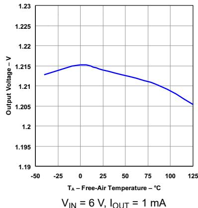
図 5-4. Output Voltage vs Temperature
