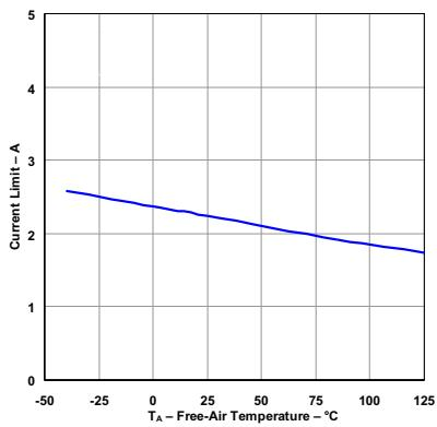
図 5-15. Current Limit vs Temperature
