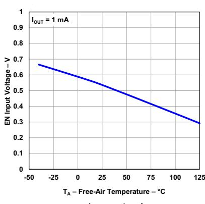
図 5-11. EN Threshold (Off to On) vs Temperature
