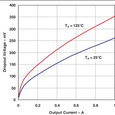
図 5-1. Dropout Voltage vs Output Current
