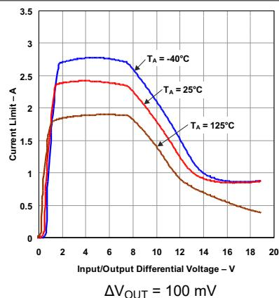
図 5-14. Current Limit vs Input/Output Differential Voltage
