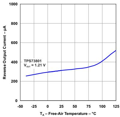
図 5-17. Reverse Output Current vs Temperature
