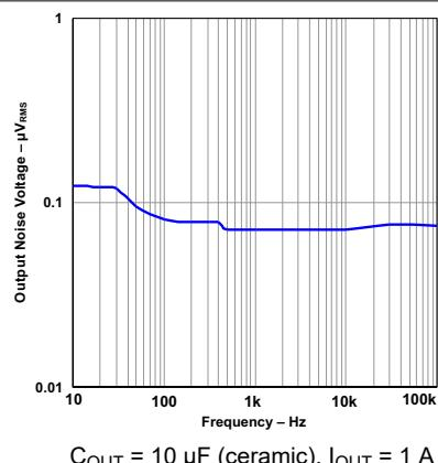
図 5-20. Output Noise Voltage vs Frequency
