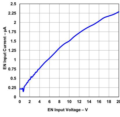
図 5-10. EN Input Current vs EN Input Voltage
