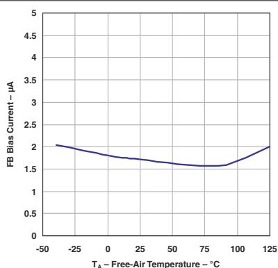
図 5-13. Fb Bias Current vs Temperature
