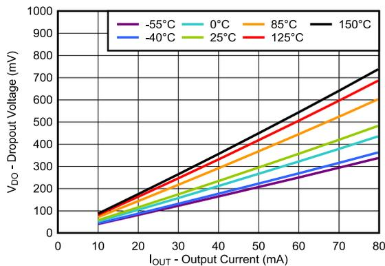
5-11. TPS71433 Dropout Voltage vs Output Current (New Chip)
