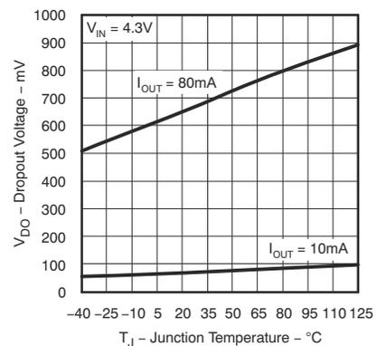
5-12. TPS71433 Dropout Voltage vs Junction Temperature (Legacy Chip)
