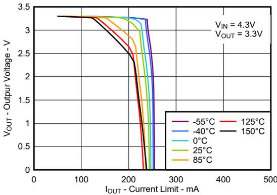
5-19. TPS71433  $V_{OUT}$  vs Current Limit (New Chip)
