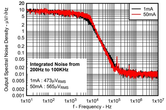
5-16. TPS71433 Output Spectral Noise Density vs Frequency (New Chip)
