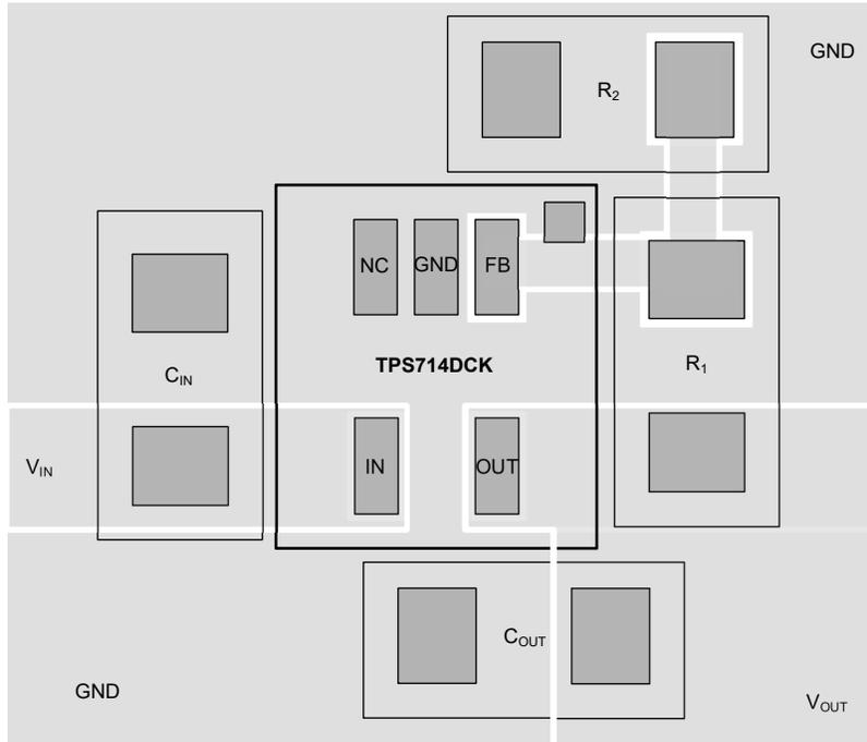
図 7-12. Example Layout for the TPS714DCK
