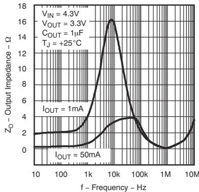
5-17. TPS71433 Output Impedance vs Frequency (Legacy Chip)
