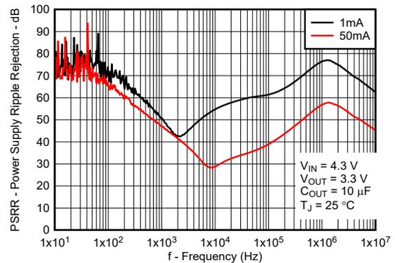
5-22. TPS71433 Power-Supply Ripple Rejection vs Frequency (New Chip)
