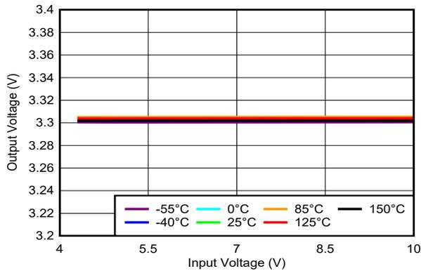
5-3. TPS71433 Output Voltage vs Input Voltage (New Chip)
