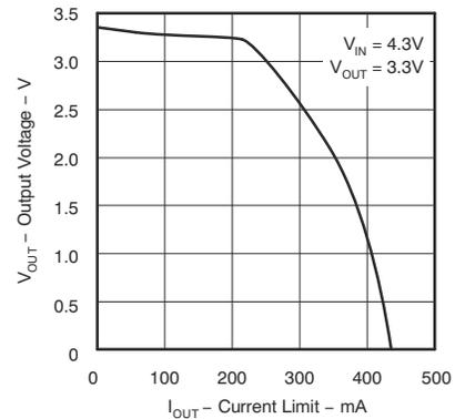
5-18. TPS71433  $V_{OUT}$  vs Current Limit (Legacy Chip)
