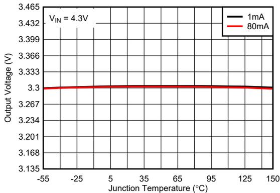
5-5. TPS71433 Output Voltage vs Junction Temperature (New Chip)
