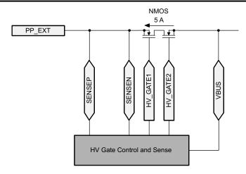
図 9-21. External HV Switch as a Sink without RSENSE
