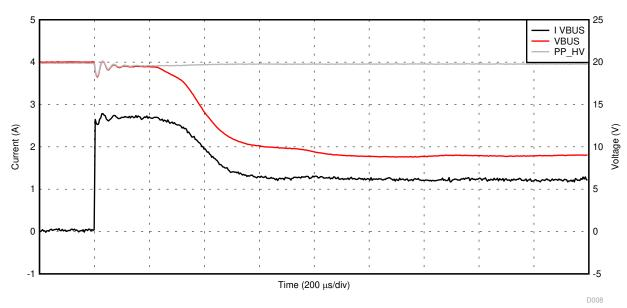
図 9-19. PP\_HV Current Limit Response With a Soft Short (7 Ω)
