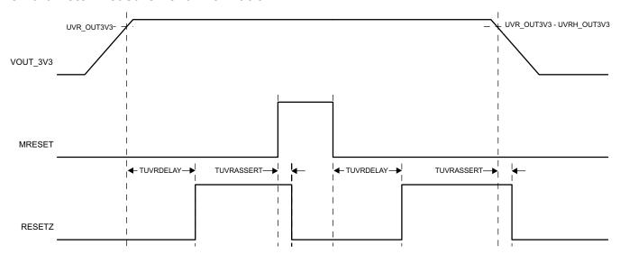
図 8-1. RESETZ Assertion Timing
