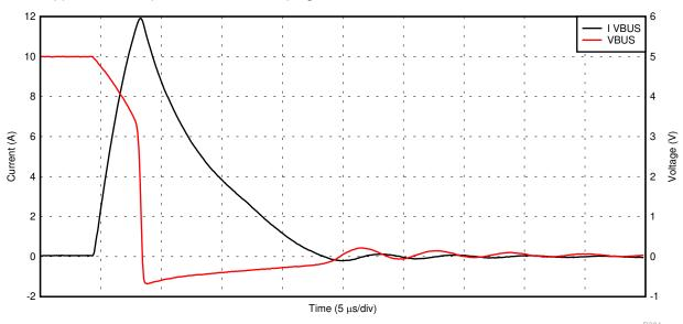
図 9-13. PP 5V0 Current Limit With a Hard Short
