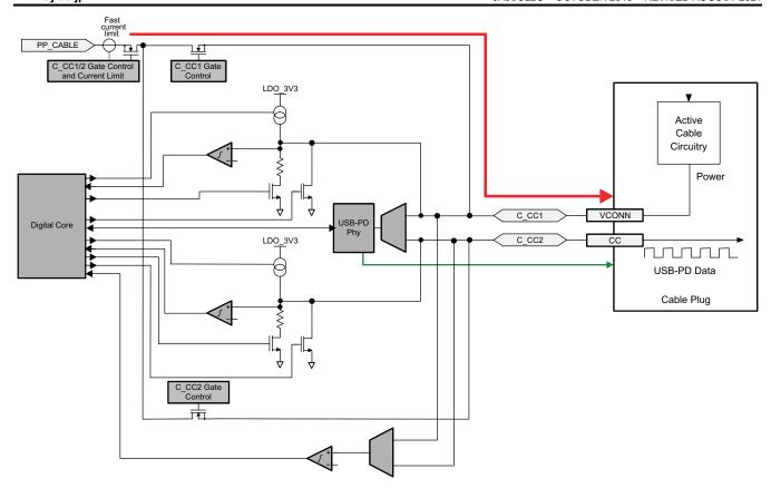
図 9-30. Port C\_CC1 and C\_CC2 Reverse Orientation Power from PP\_CABLE
