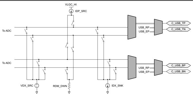
図 9-39. BC1.2 Detection Circuitry
