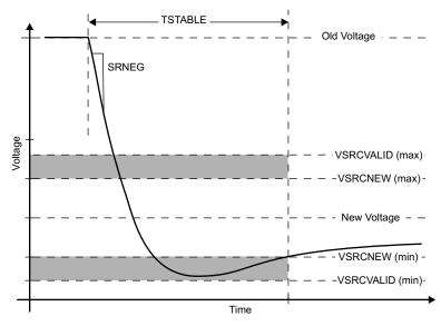
図 9-26. Negative Voltage Transition on VBUS
