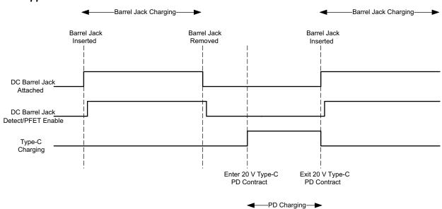
図 10-6. DC Barrel Jack and Type-C PD Charging Hand-Off
