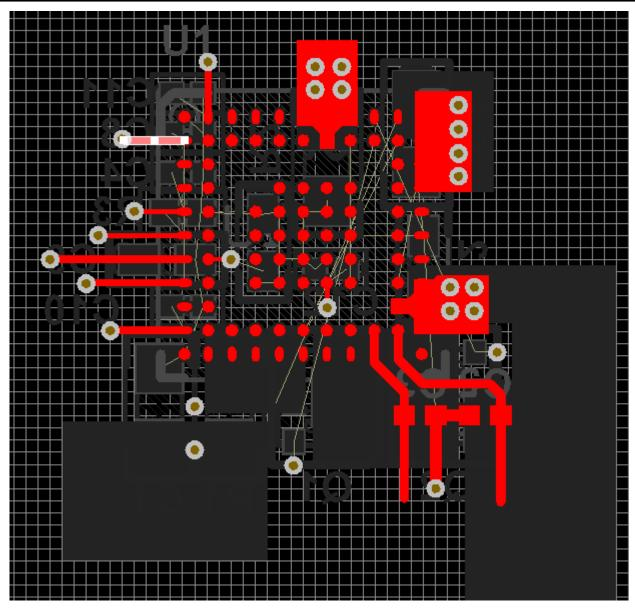
図 12-13. Top Layer Component Routing
