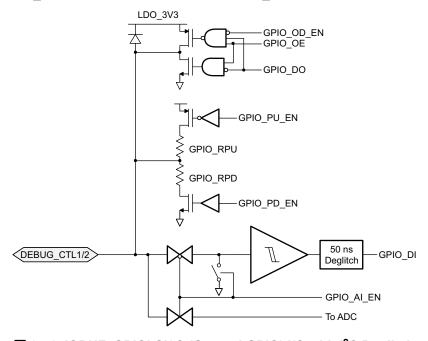
図 9-46. IOBUF\_GPIOLSI2C (General GPIO) I/O with I<sup>2</sup>C Deglitch
