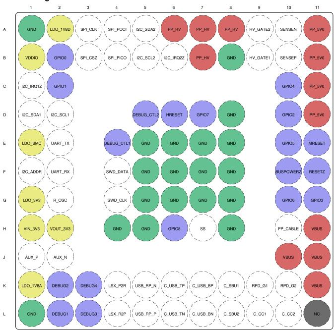
図 6-1. ZQZ and ZBH Package 96-Pin BGA MicroStar Junior and NFBGA Top View
