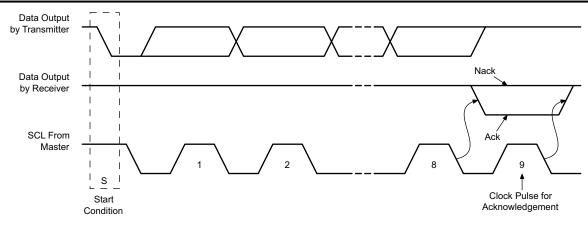
図 9-64. I<sup>2</sup>C Acknowledgment
