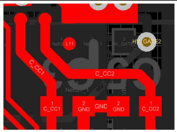
図 12-12. CC1 and CC2 Capacitor Routing
