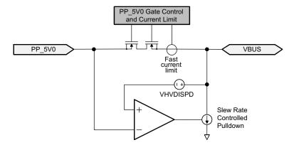
図 9-27. PP\_5V0 Slew Rate Control
