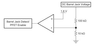
図 10-5. Barrel Jack Detect Comparator
