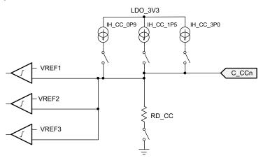
図 9-9. Plug and Orientation Detection Block
