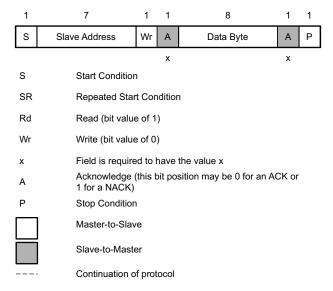
図 9-67. I<sup>2</sup>C Read/Write Protocol Key
