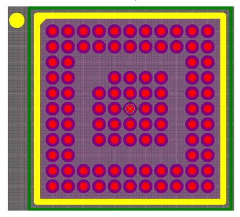
図 12-1. Top View Standard TPS65983B Footprint (Circular Pads)
