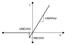
図 9-16. Internal HV Switch I-V Curve as a Source
