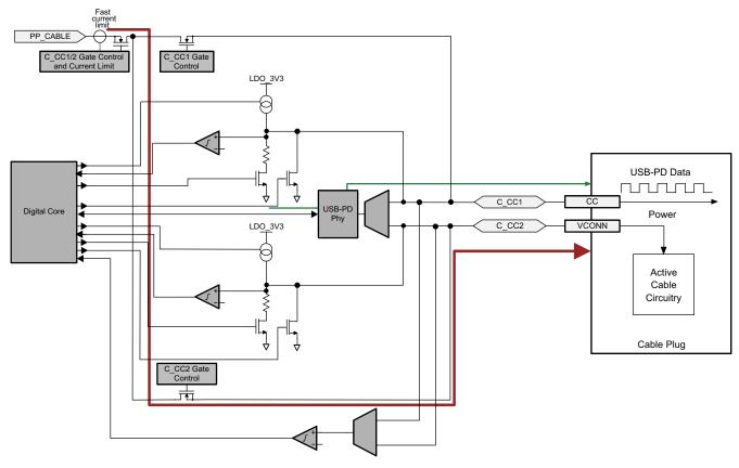
図 9-29. Port C\_CC1 and C\_CC2 Normal Orientation Power from PP\_CABLE
