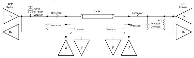
図 9-8. Example USB-PD Multi-Drop Configuration
