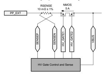
図 9-20. External HV Switch as a Sink with RSENSE
