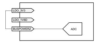
図 9-22. BUSPOWERZ Configured to Disable Power from VBUS
