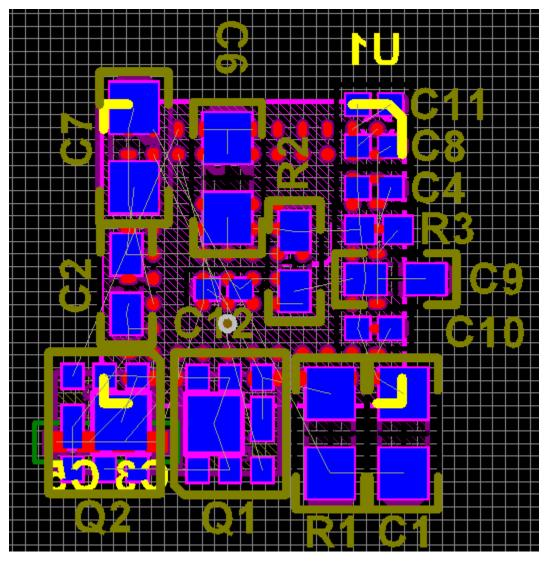
図 12-7. Example Layout (Bottom View in 2-D)
