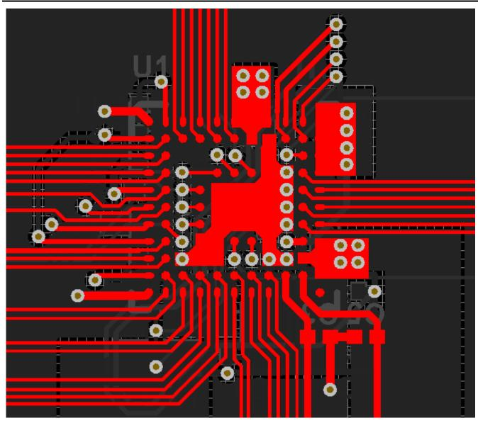
図 12-17. Final Routing and GND Pour (Top Layer)
