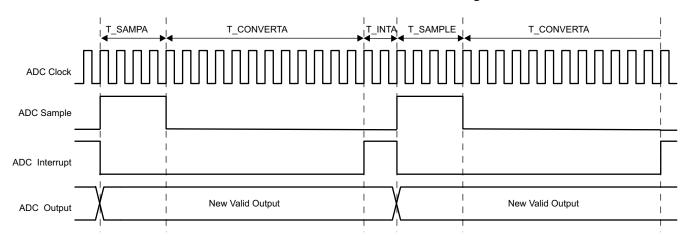
図 8-3. ADC Repeated Conversion Timing
