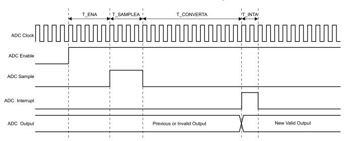
図 8-2. ADC Enable and Conversion Timing
