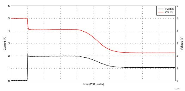
図 9-15. PP\_5V0 Current Limit With a Soft Short (2 Ω)
