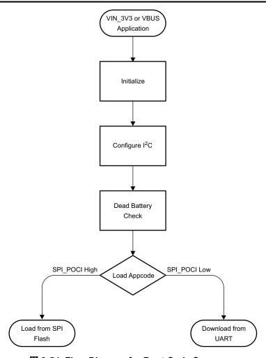
図 9-54. Flow Diagram for Boot Code Sequence
