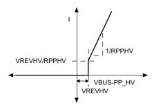
図 9-17. Internal HV Switch I-V Curve as a Sink
