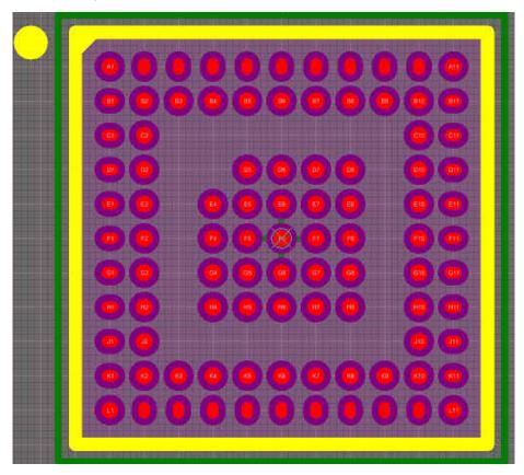
図 12-3. Top View Alternate TPS65983B Footprint (Oval Pads)
