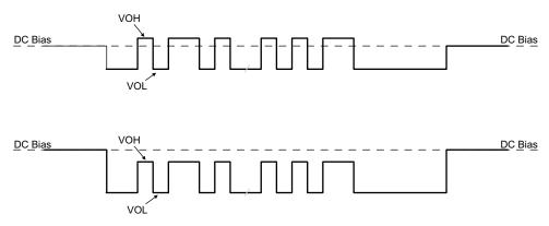
図 9-6. TX Driver Transmission with DC Bias
