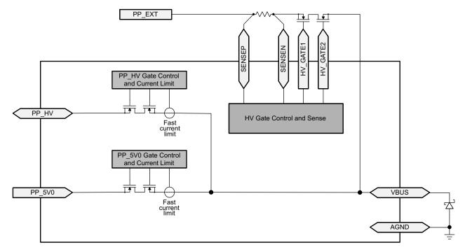
図 11-1. Schottky on VBUS for Current Surge Protection
