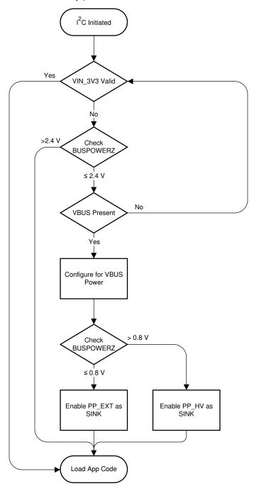
図 9-56. Dead-Battery Condition Flow Diagram
