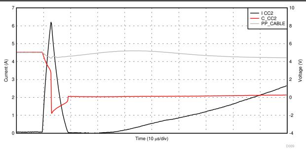
図 9-31. PP\_CABLE to C\_CCn Current Limit With a Hard Short
