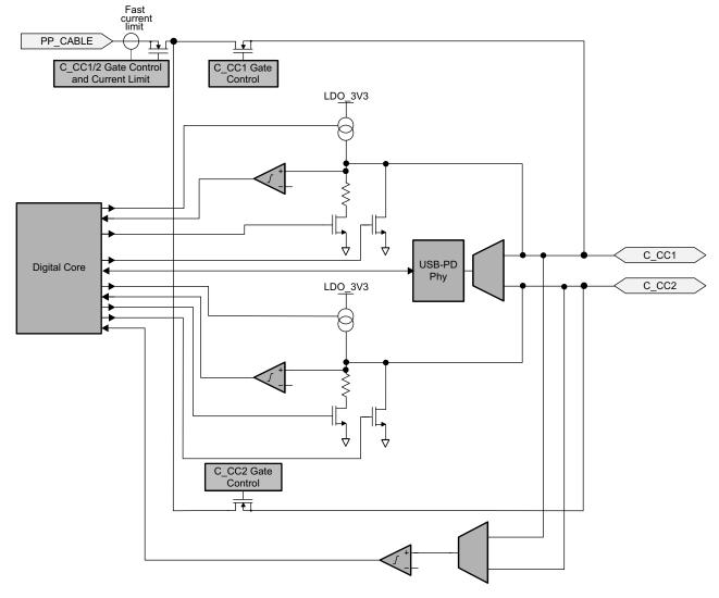
図 9-1. USB-PD Physical Layer and Simplified Plug and Orientation Detection Circuitry
