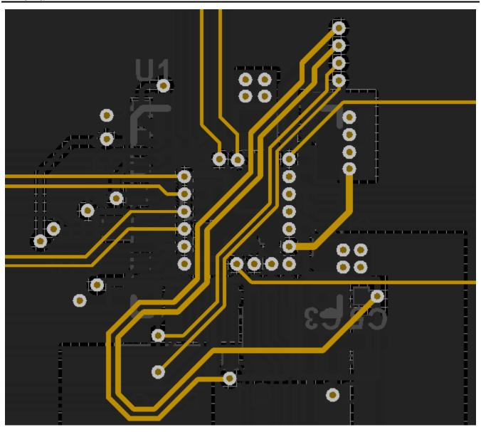
図 12-18. Final Routing (Inner Signal Layer)
