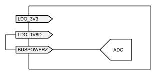
図 9-23. BUSPOWERZ Configured with PP\_HV as Input Power Path
