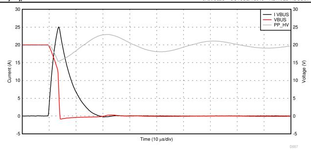
図 9-18. PP\_HV Current Limit Response With a Hard Short
