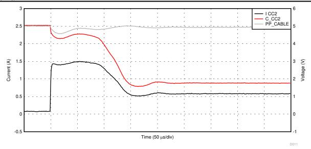
図 9-33. PP\_CABLE to C\_CCn Current Limit Response With a Soft Short (2 Ω)
