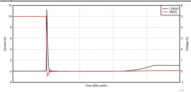
図 9-14. PP\_5V0 Current Limit With a Hard Short (Extended Time Base)
