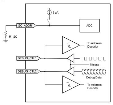
図 9-68. I<sup>2</sup>C Address Decode
