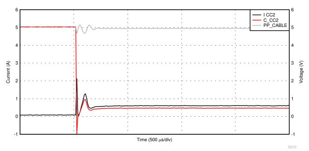
図 9-32. PP\_CABLE to C\_CCn Current Limit With a Hard Short (Extended Time Base)
