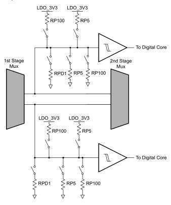
図 9-36. Port Detect and Pullup and Pulldown
