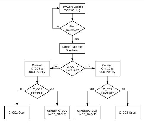
図 9-28. Port C\_CC and VCONN Connection Flow
