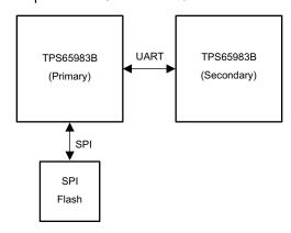
図 9-61. Primary and Secondary TPS65983B Sharing a Single Flash
