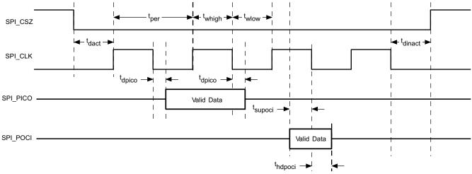
図 8-5. SPI Controller Timing
