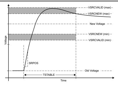
図 9-25. Positive Voltage Transition on VBUS
