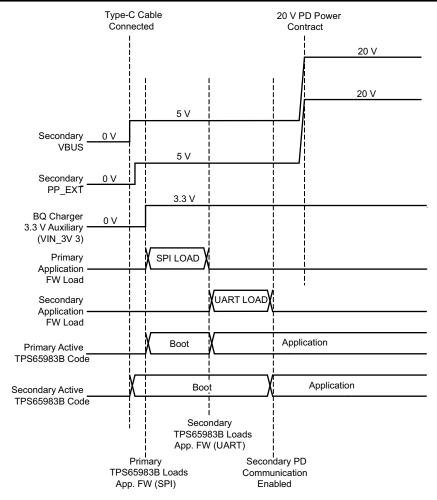
図 10-8. Secondary TPS65983B Dead Battery Sequence
