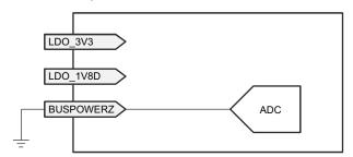
図 9-24. BUSPOWERZ Configured with PP\_EXT as Input Power Path
