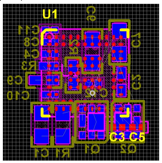
図 12-6. Example Layout (Top View in 2-D)
