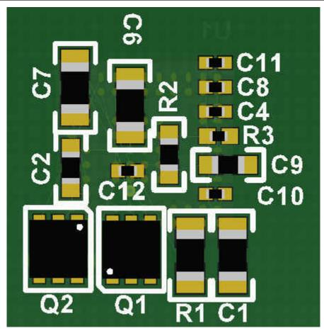
図 12-9. Example Layout (Bottom View in 3-D)
