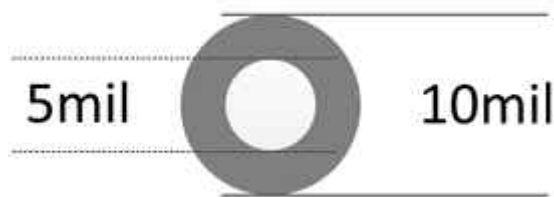
✎ 12-2. Under Ball Recommended Via Size
