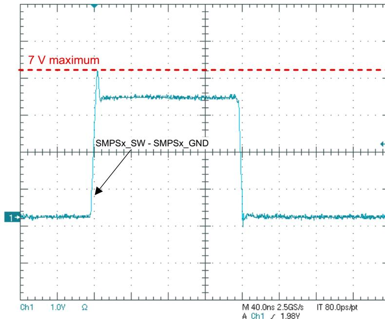
Measure across the low-side FET (SMPSx\_SW – GND) as close to the IC as possible. The preferred measurement is with a differential probe. The negative side of the probe should be at GND and the positive side of the probe should measure SMPSx\_SW. As shown in this image, the voltage across the low-side FET should not exceed 7 V. Repeat the measurement for all SMPSs in use.
