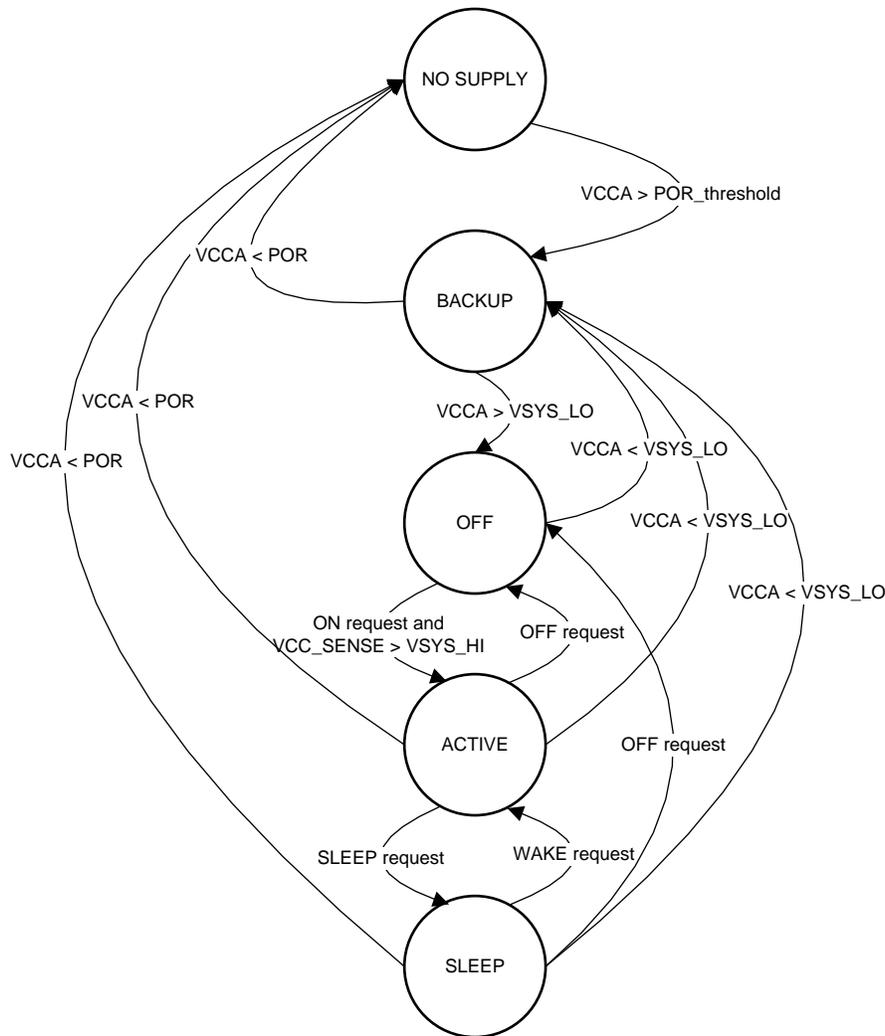
☒ 5-2. State Diagram for the Power Control State-Machine
