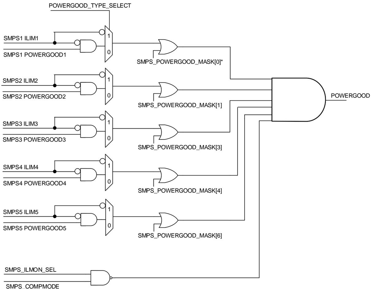
\*When operating in dual phase, SMPS\_POWERGOOD\_MASK[0] controls the monitoring of SMPS12. SMPS\_POWERGOOD\_MASK[1] is masked internally with dual phase operation.
