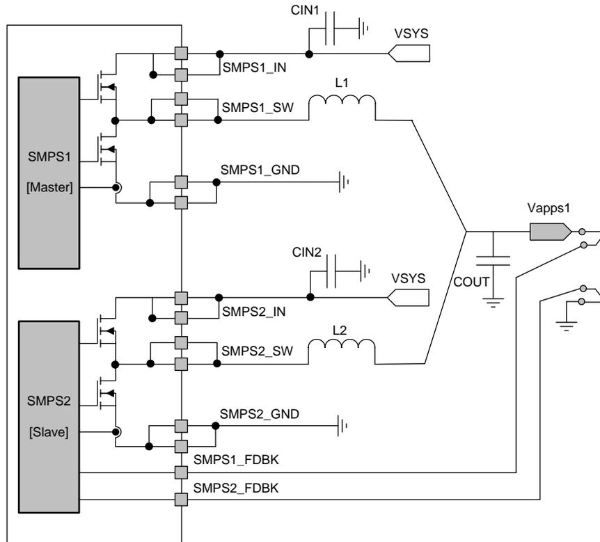
图 5-14. SMPS1&2 Dual-Phase Configuration
