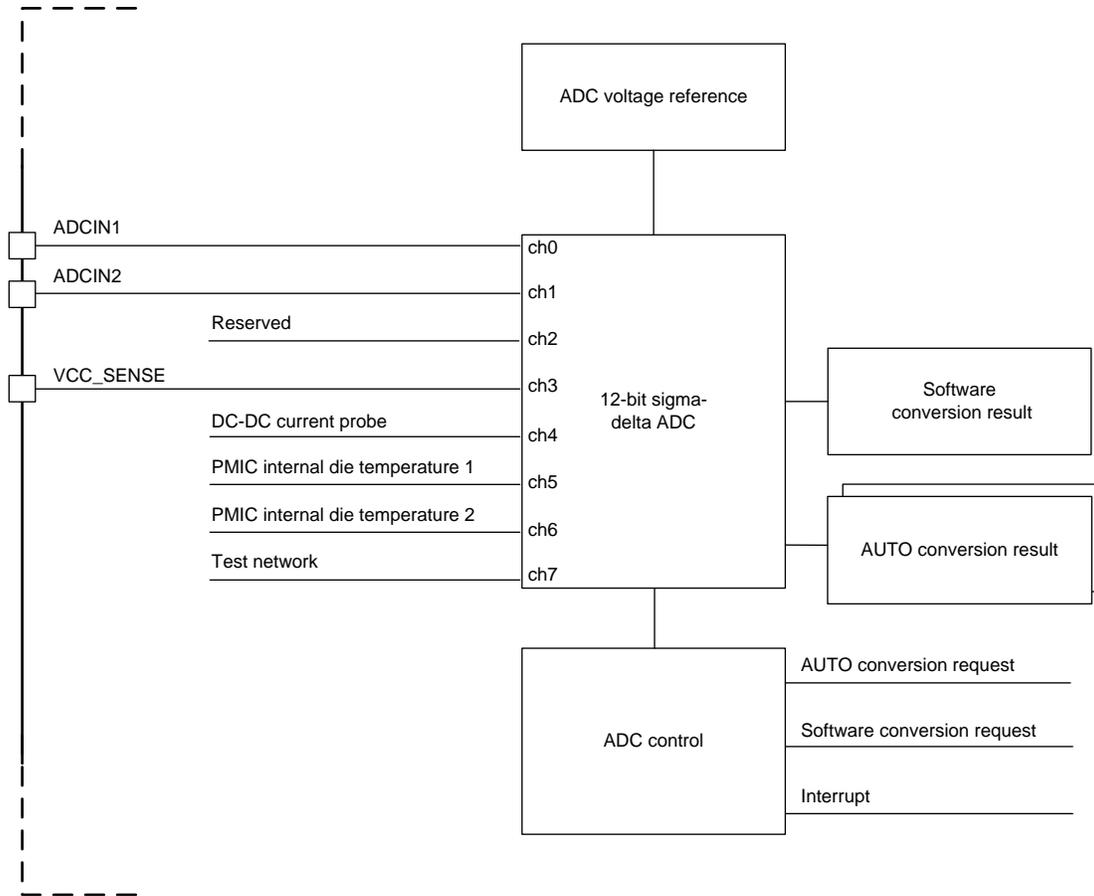
图 5-15. Block Diagram of the GPADC
