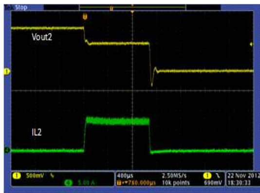
Figure 29. Over Current Protection, Buck 2
