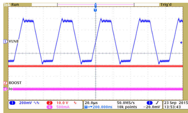
Figure 8-8. No Load, 22-kHz Tone Output
