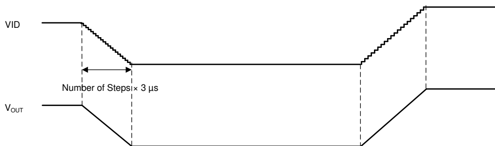
図 7-19. DVS Timing Diagram I (BUCKx_DECAY = 0)
