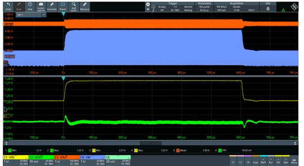
$V_{IN} = 2.4V \sim 5.5V$   $V_{OUT} = 1.2V$  負荷 = 6A
