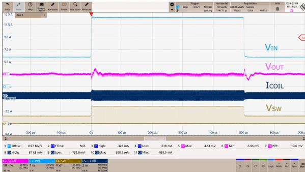
$V_{IN} = 2.4V \sim 5.5V$   $V_{OUT} = 1.2V$  負荷 = 10mA
