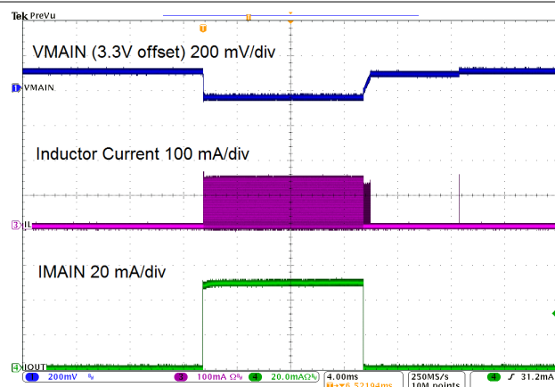
TPS610981 V_{IN} = 2.5 V I_{(SUB)} = 0 mA MODE = L I_{(MAIN)} = 0 mA to 50 mA, 5 \mu s rising/falling edge
