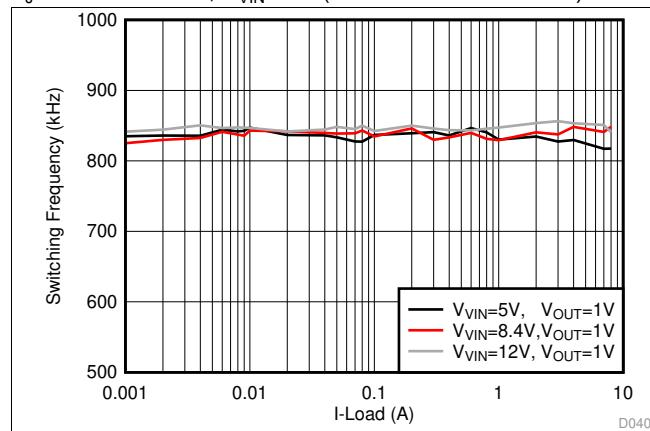
図 25.  $F_{\text{sw}}$  Load Regulation, FCCM,  $F_{\text{sw}} = 800 \text{ kHz}$
