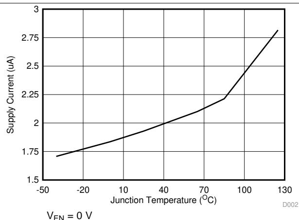
図 2. Shutdown Current vs Temperature
