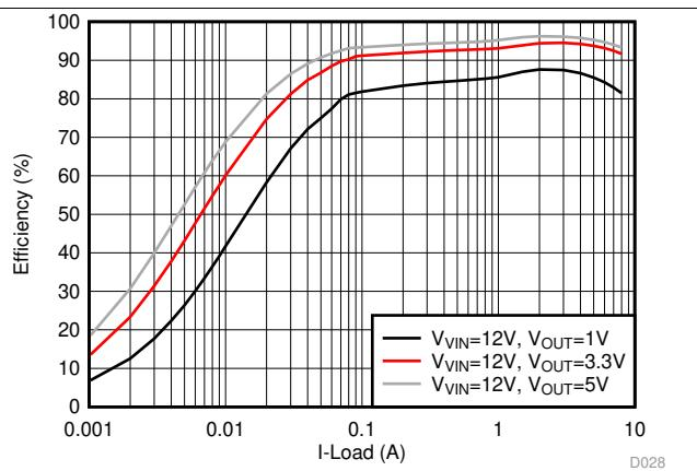
図 14. Efficiency, OOA-mode,  $F_{\text{SW}} = 600 \text{ kHz}$
