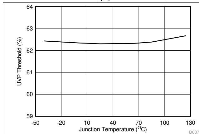
図 9. UVP Threshold vs Junction Temperature
