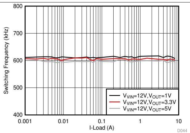
図 26.  $F_{\text{sw}}$  Load Regulation, FCCM,  $F_{\text{sw}} = 600 \text{ kHz}$
