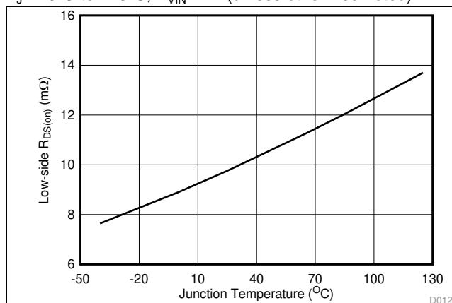
図 7. Low-Side  $R_{\text{DS}(\text{on})}$  vs Junction Temperature
