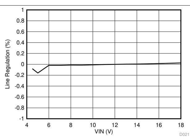
图 36. Line Regulation,  $I_{OUT} = 8\text{ A}$
