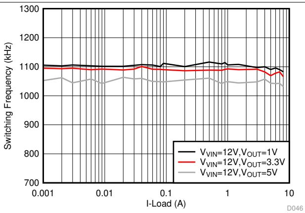
図 28.  $F_{\text{sw}}$  Load Regulation, FCCM,  $F_{\text{sw}} = 1 \text{ MHz}$
