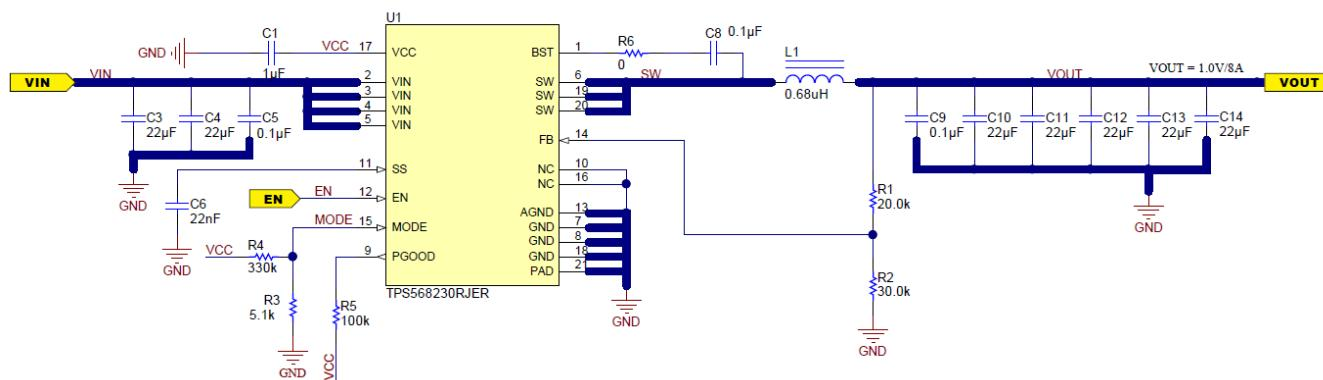
**図 30. 1-V, 8-A Reference Design with Eco-mode,  $F_{SW} = 600$  kHz**
