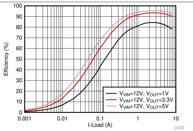
図 18. Efficiency, FCCM,  $F_{\text{SW}} = 1 \text{ MHz}$
