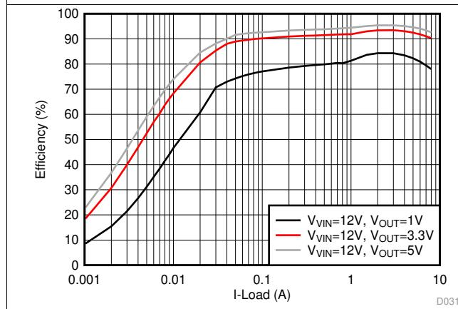
図 17. Efficiency, OOA-mode,  $F_{\text{SW}} = 1 \text{ MHz}$
