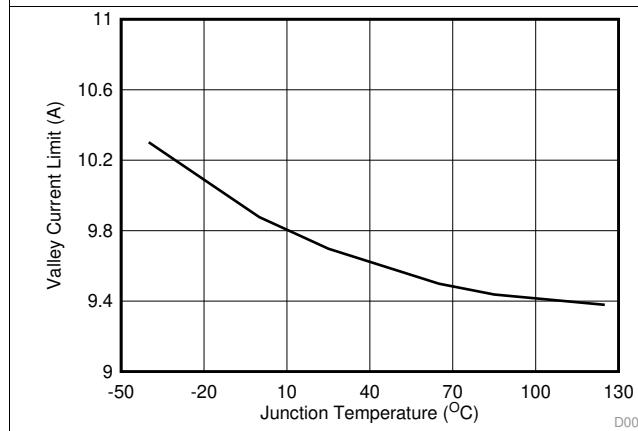
図 11. Valley Current Limit vs Junction Temperature
