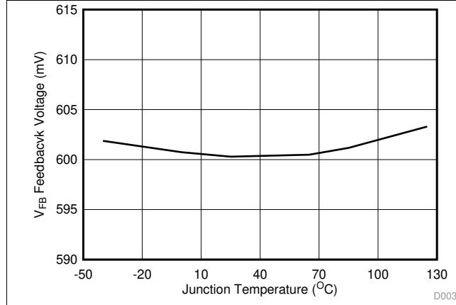
図 3. Feedback Voltage vs Junction Temperature
