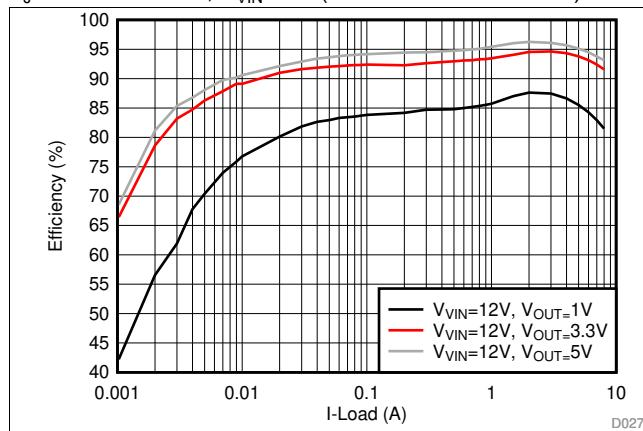
図 13. Efficiency, Eco-mode,  $F_{\text{SW}} = 600 \text{ kHz}$
