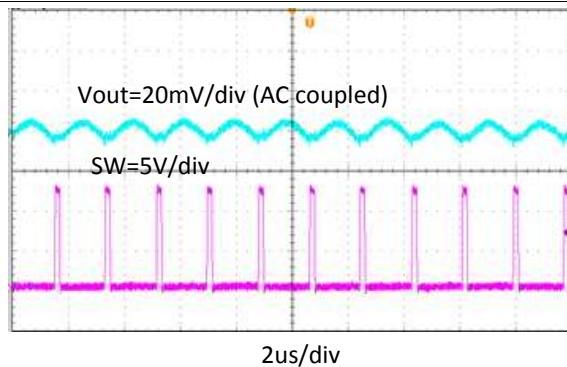
図 38. Output Voltage Ripple,  $I_{OUT} = 8 \text{ A}$
