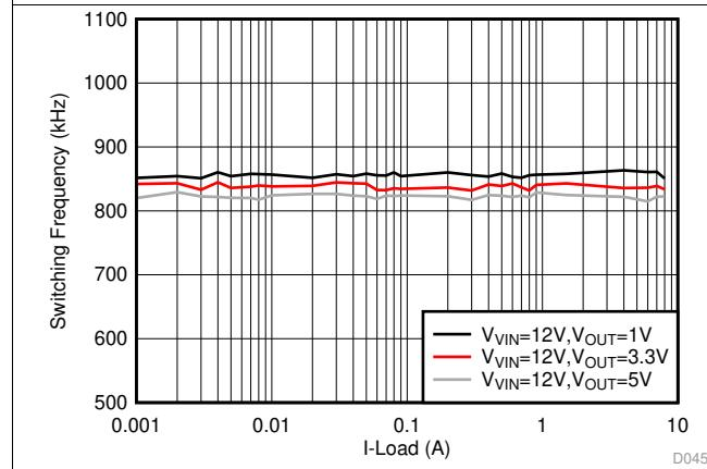
図 27.  $F_{\text{sw}}$  Load Regulation, FCCM,  $F_{\text{sw}} = 800 \text{ kHz}$
