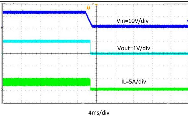
図 42. Start Up Relative to  $V_{IN}$  Falling,  $I_{OUT} = 4 \text{ A}$
