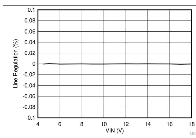
图 35. Line Regulation,  $I_{OUT} = 0.01\text{ A}$
