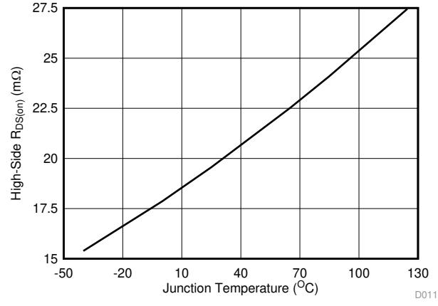
図 6. High-Side RDS(on) vs Junction Temperature
