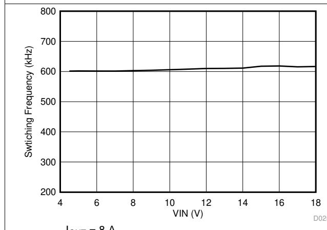
图 33. Switching Frequency vs Input Voltage
