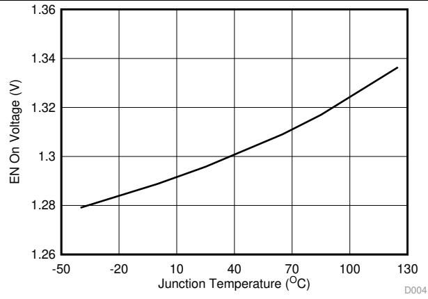
図 4. Enable On Voltage vs Junction Temperature
