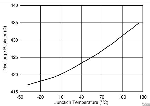
図 10. Discharge Resistor vs Junction Temperature
