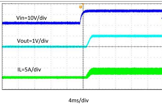
図 41. Start Up Relative to  $V_{IN}$  Rising,  $I_{OUT} = 4 \text{ A}$
