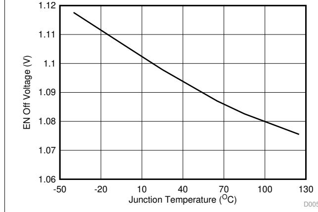
図 5. Enable Off Voltage vs Junction Temperature
