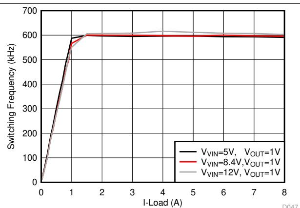
图 34. Switching Frequency vs Output Load
