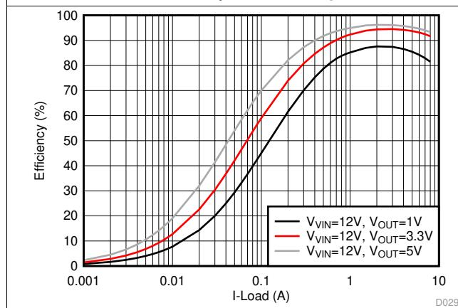
図 15. Efficiency, FCCM,  $F_{\text{SW}} = 600 \text{ kHz}$
