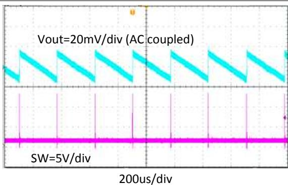
図 37. Output Voltage Ripple,  $I_{OUT} = 0.01 \text{ A}$
