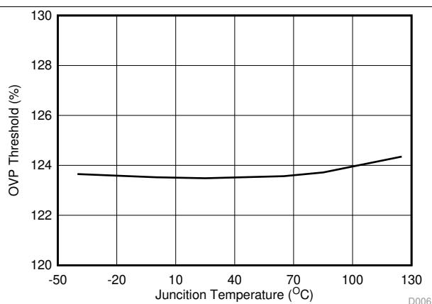
図 8. OVP Threshold vs Junction Temperature
