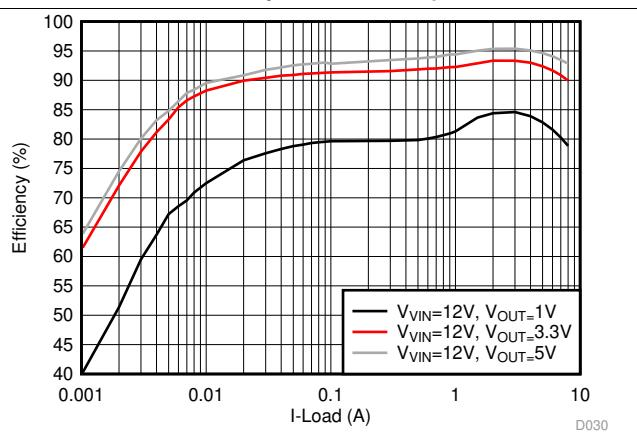
図 16. Efficiency, Eco-mode,  $F_{\text{SW}} = 1 \text{ MHz}$
