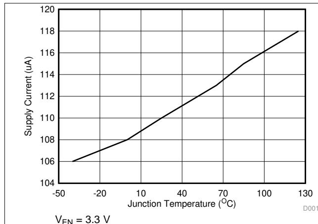
図 1. Supply Current vs Junction Temperature
