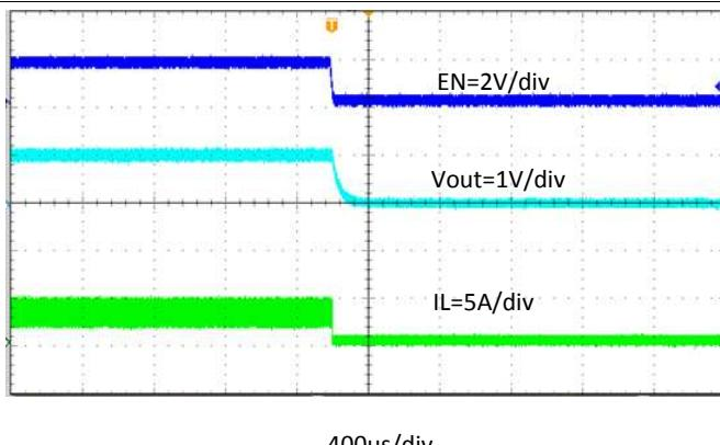
図 40. Shut-down Through EN,  $I_{OUT} = 4 \text{ A}$
