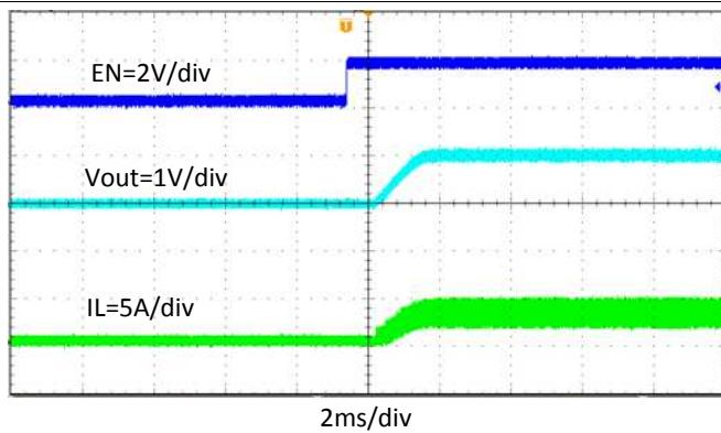
図 39. Start-Up Through EN,  $I_{OUT} = 4 \text{ A}$
