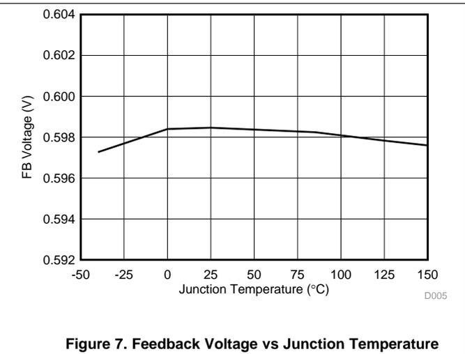
Figure 7. Feedback Voltage vs Junction Temperature
