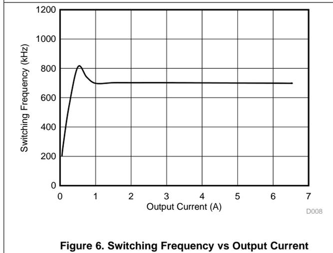
Figure 6. Switching Frequency vs Output Current
