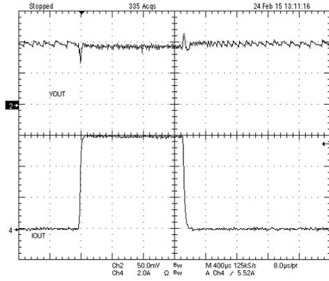
**Figure 24. Load Transient**
