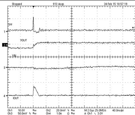
**Figure 28. Skip Mode (Inductor Current)**
