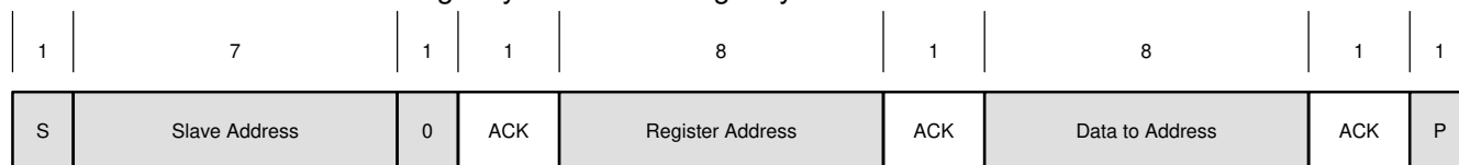
FIG 7-11. Single-byte Write
