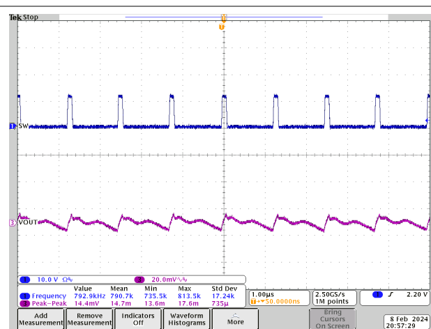
Figure 7-15. Output Voltage Ripple, 800kHz FCCM, No load, PVIN = 12V, VOUT = 1.1V
