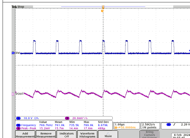
図 7-14. Output Voltage Ripple, 800kHz FCCM, 40A Load, PVIN = 12V, VOUT = 1.1V
