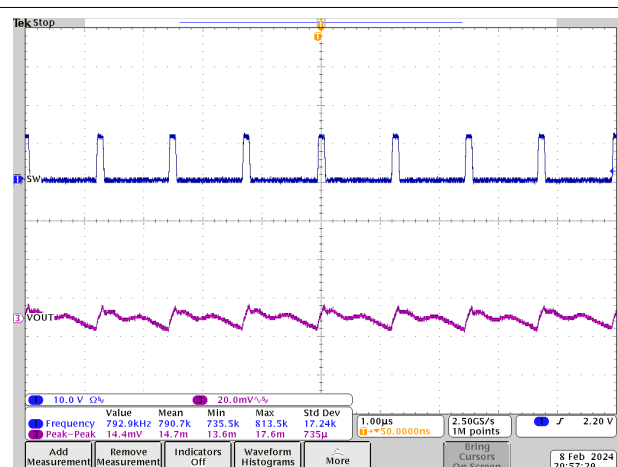
図 7-15. Output Voltage Ripple, 800kHz FCCM, No load, PVIN = 12V, VOUT = 1.1V
