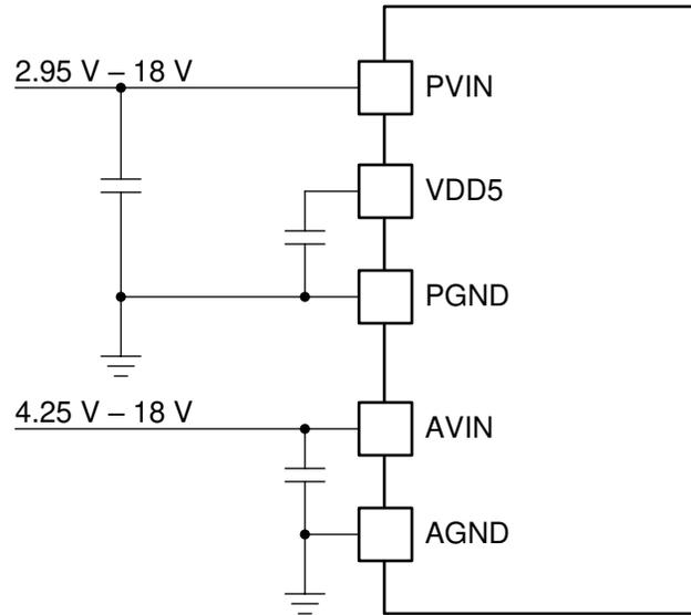
Figure 7-2. TPS546B24A Separate PVIN and AVIN connections
