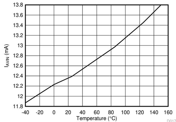
6-10. Non-Switching Input Current ( $I_{AVIN}$ ) vs Junction Temperature
