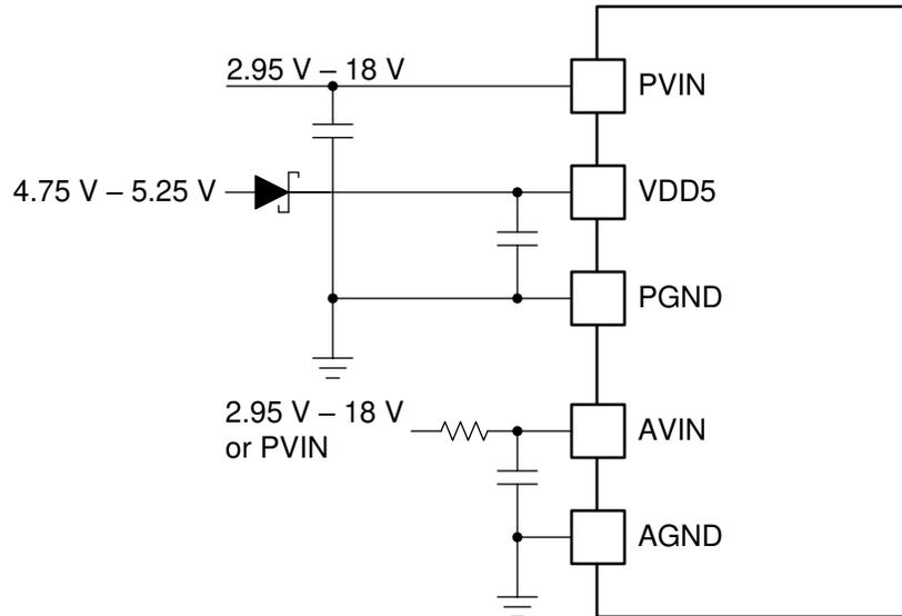
FIG 7-4. TPS546B24A Separate PVIN, AVIN, and VDD5 Connections
