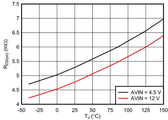
6-7. High-Side MOSFET On-Resistance ( $R_{DS(on)}$ ) vs Junction Temperature
