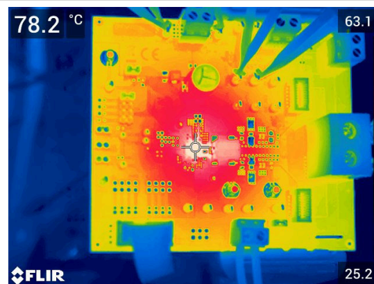
图 8-22. Thermal Characteristics, 600 kHz FCCM, External 5-V Bias, 35-A Load
