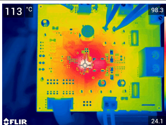
图 8-25. Thermal Characteristics, 1.2-MHz FCCM, Internal LDO, 35-A Load
