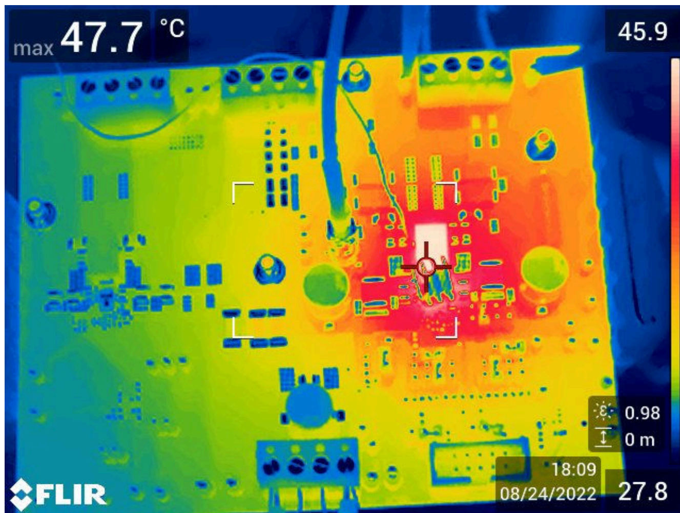
図 7-24. Thermal Image at 25°C Ambient
