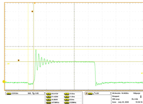
図 6-22. Switch Node Ringing and Dead-Time at 10-A Output Current
