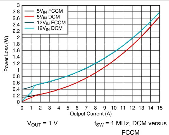
**6-4. Power Loss vs Output Current**
