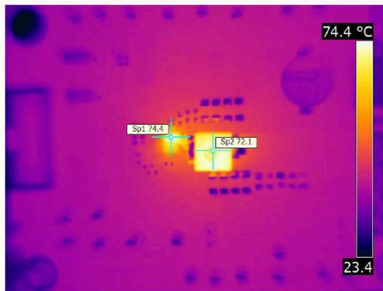
$V_{IN} = 12\text{ V}$        $V_{OUT} = 5\text{ V}$        $f_{SW} = 0.6\text{ MHz}$
