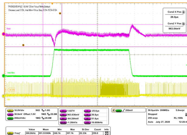
6-26. Load Transient 2 A to 12 A to 2 A at 20 A/ \mu s
