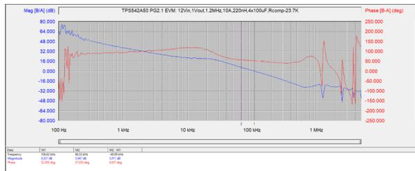
图 8-4. Bode Plot at 10-A Output Current
