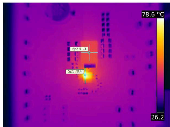
图 6-13. Thermal Image at 15-A Output Current
