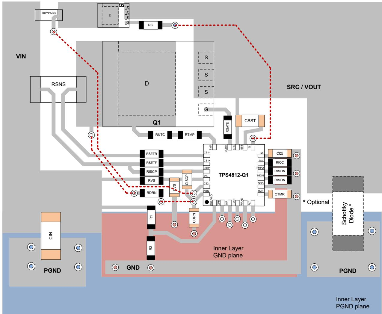
図 9-20. Typical PCB Layout Example of TPS4812-Q1
