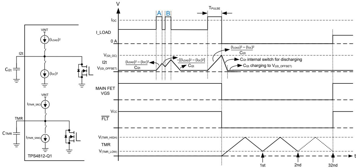
図 8-9. I<sup>2</sup>t-Based Overcurrent Protection With Auto-Retry
