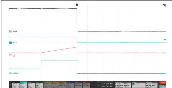
図 9-8. I<sup>2</sup>T based Overcurrent Response of TPS4812-Q1 EVM for 6A to 16A Load Step
