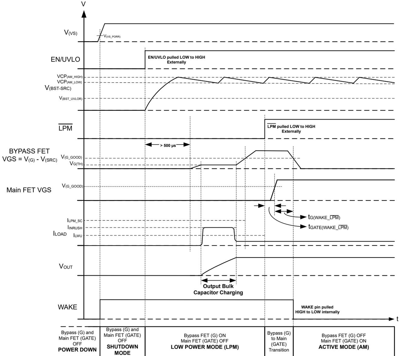
8-16. State Transition Timing Diagram With LPM Trigger
