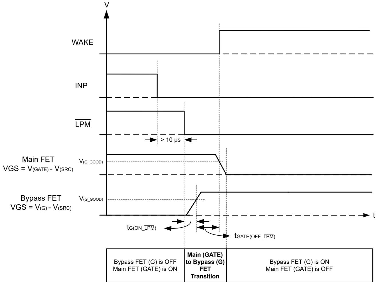
図 7-3. Active Mode to Low Power Mode by  $\overline{LPM}$  Trigger
