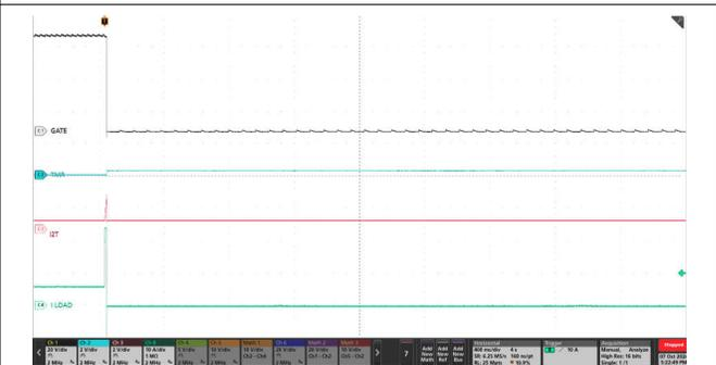
図 9-11. Latch-Off Response of TPS4812-Q1 for an I<sup>2</sup>T-Based Overcurrent Fault
