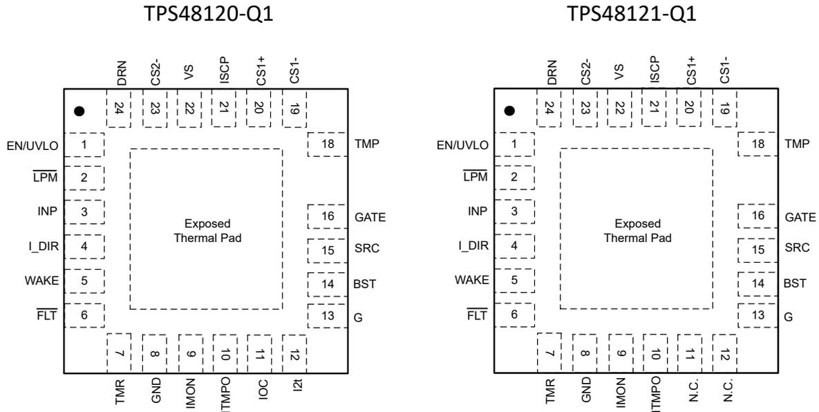
図 5-1. RGE Package, 23-Pin VQFN (Transparent Top View)
