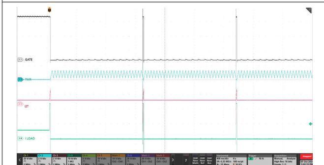
図 9-10. Auto-Retry Response of TPS4812-Q1 for an I<sup>2</sup>T-Based Overcurrent Fault
