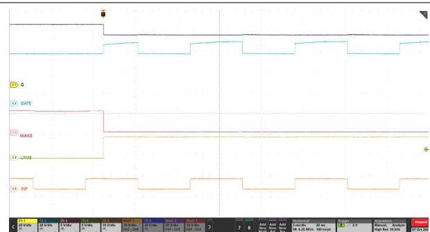
図 9-7. With \overline{\text{LPM}} = Low to High, INP Gained Control on GATE (VIN = 48V, No Load)
