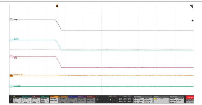
9-15. GATE Turn-OFF During Input Reverse Battery Fault
