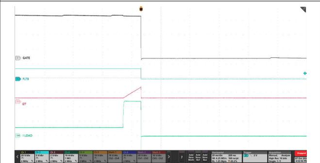
図 9-9. I<sup>2</sup>T based Overcurrent Response of TPS4812-Q1 EVM for 6A to 23A Load Step
