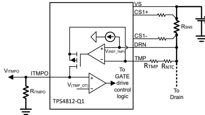
**Fig 8-12. NTC-Based Temperature Sensing and Monitoring Output**
