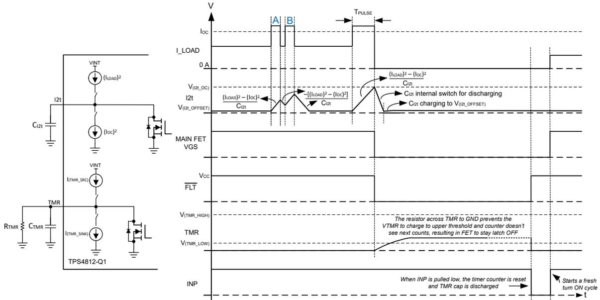
8-10. I<sup>2</sup>t-Based Overcurrent Protection With Latch-Off
