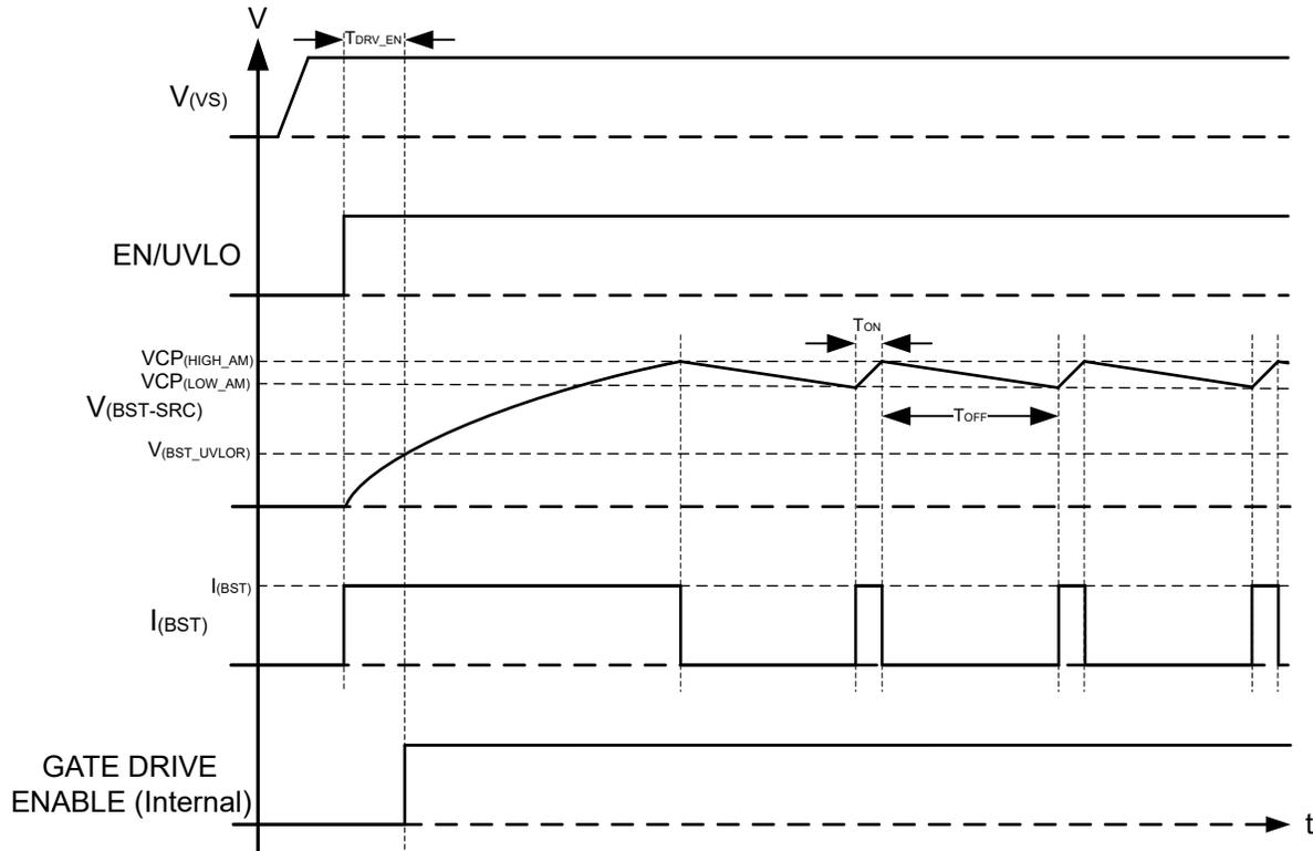
図 8-2. Charge Pump Operation
