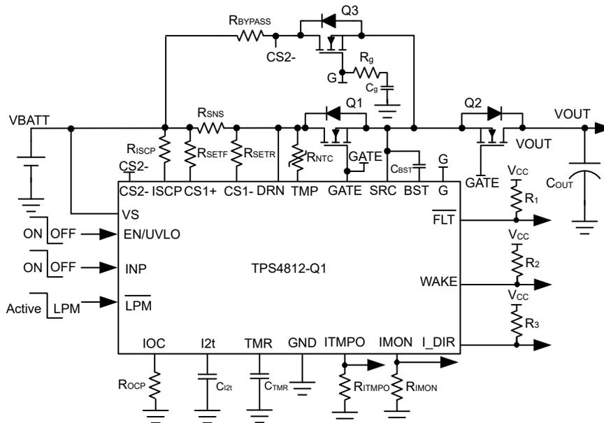
**☒ 8-6. TPS4812-Q1 Application Circuit for Capacitive Load Driving Using Low-Power Bypass FET (Q<sub>3</sub>) and Series Resistor (R<sub>BYPASS</sub>)**
