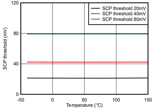
图 5-6. Short-Circuit Threshold (V(SCP)) vs Temperature
