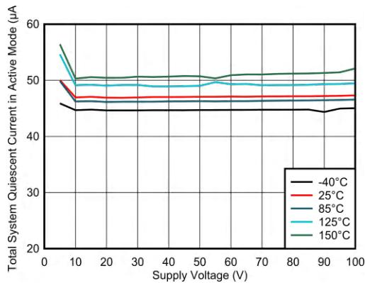
图 5-2. Operating Quiescent Current in Active Mode vs Supply Voltage
