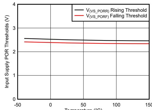
**图 5-8. Input Supply POR Thresholds vs Temperature**
