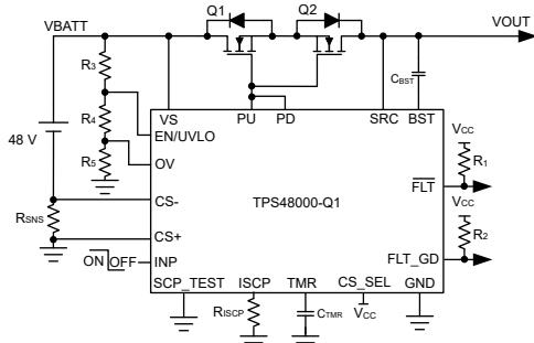
**图 7-7. TPS48000-Q1 Application Circuit With External Sense Resistor RSNS Based Low Side Current Sensing on Battery Side**
