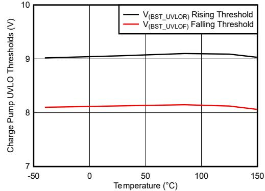
图 5-5. Charge Pump UVLO Thresholds vs Temperature
