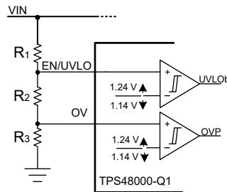
図 7-11. Programming Overvoltage and Undervoltage Protection Threshold
