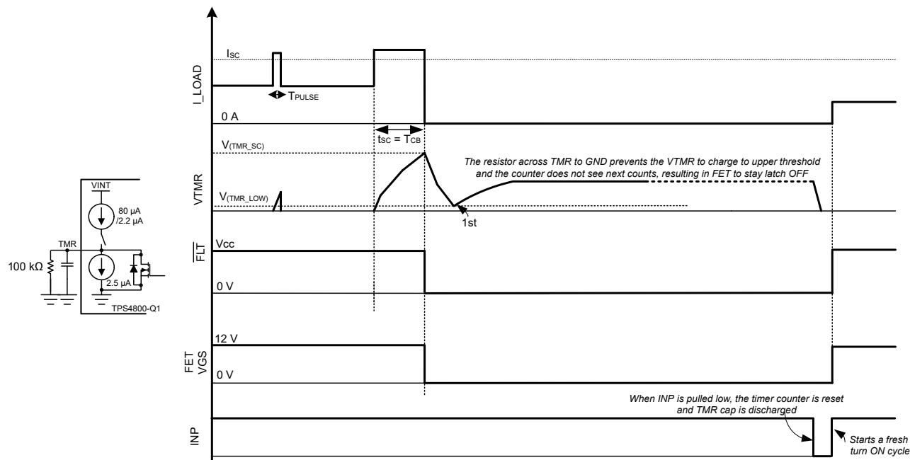
**图 7-10. Short-Circuit Protection With Latch-Off**
