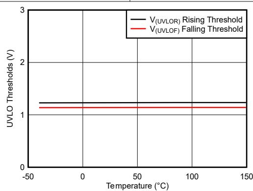
**图 5-9. Input Supply UVLO Thresholds vs Temperature**
