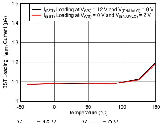
图 5-4. BST Loading Current (I(BST)) vs Temperature
