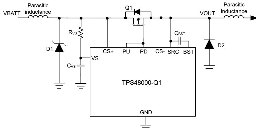
図 8-12. Circuit Implementation With Optional Protection Components For TPS48000-Q1
