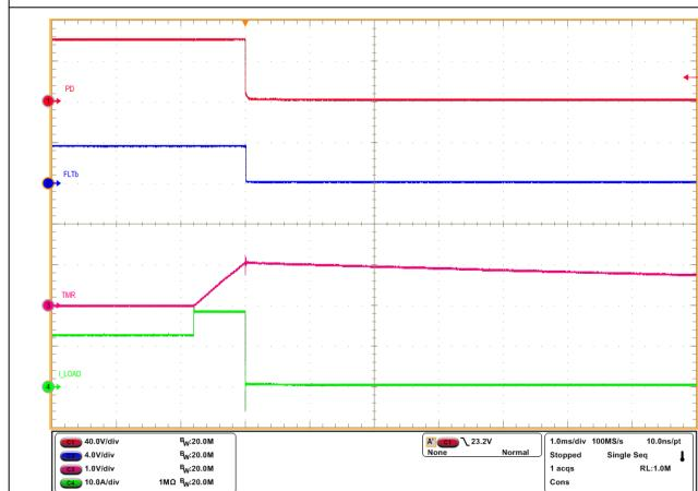
図 8-6. Overcurrent Response of TPS48000-Q1 for
