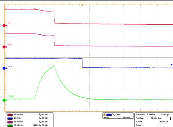
図 8-9. Output Short-Circuit Response of TPS48000-Q1 Device with 15A Shortcircuit Protection Setting and TMR = OPEN
