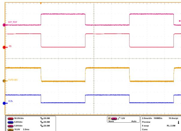
図 8-11. Short-Circuit Protection Diagnosis Test Response of TPS48000-Q1
