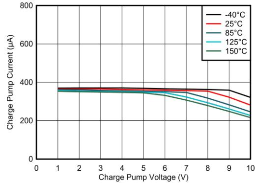
图 5-3. Charge Pump Current vs Charge Pump Voltage
