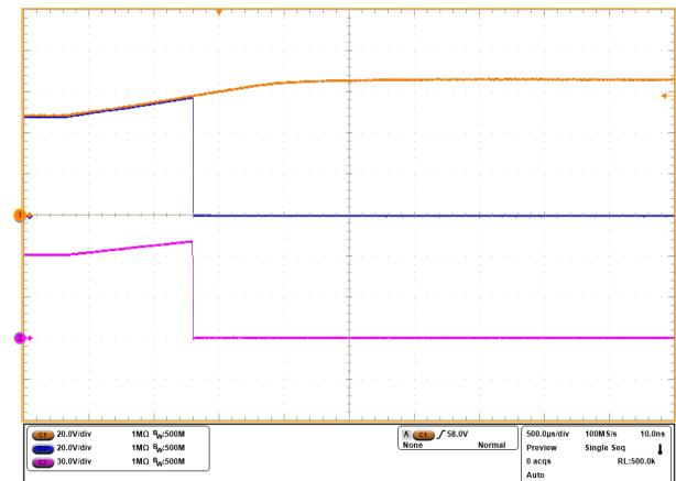
図 8-10. Overvoltage Cutoff Response of TPS48000-Q1 at 58V Level
