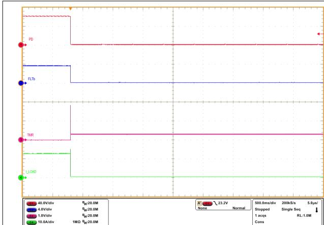
図 8-8. Latch-Off Response of TPS48000-Q1 for an Overcurrent Fault
