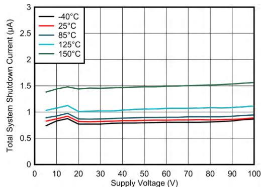
图 5-1. Shutdown Supply Current vs Supply Voltage
