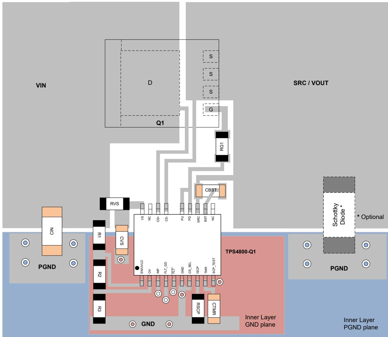
図 8-13. Typical PCB Layout Example for TPS48000-Q1 With VDS based Current Sensing
