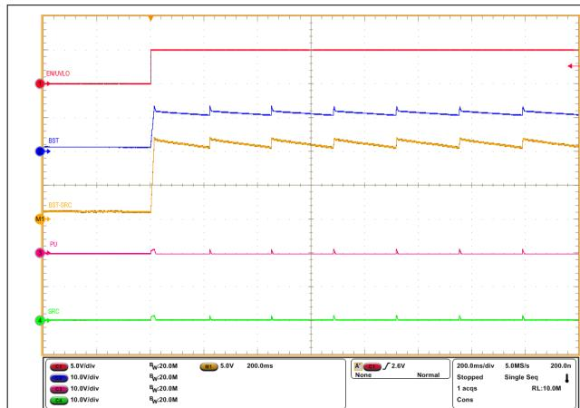
図 8-2. Start-Up Profile of Bootstrap Voltage with
