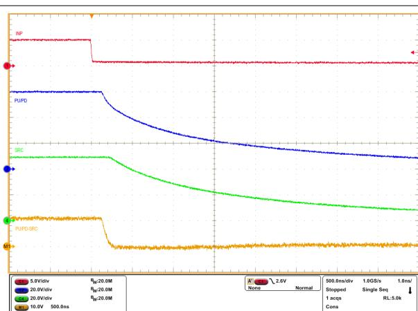
図 8-5. Turn-OFF Response of TPS48000-Q1 for INP
