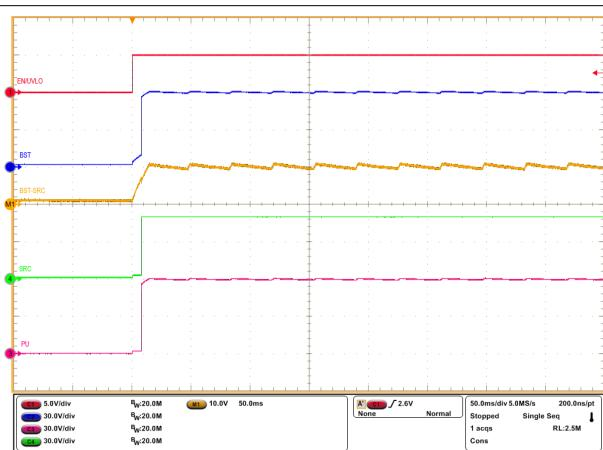
図 8-3. Start-Up Profile of Bootstrap Voltage with
