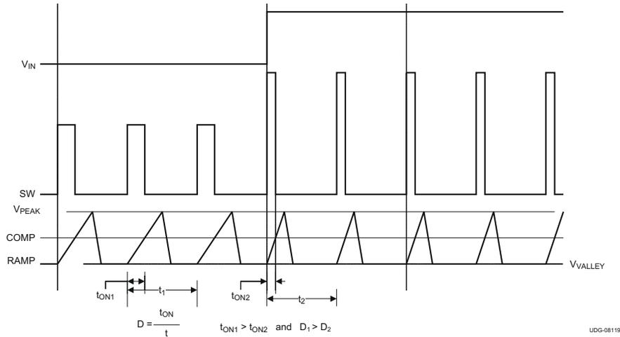
**图 7-1. Voltage Feedforward Effect on PWM Duty Cycle**
