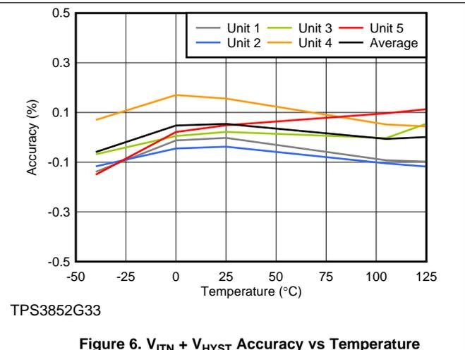
Figure 6. VITN + VHYS Accuracy vs Temperature
