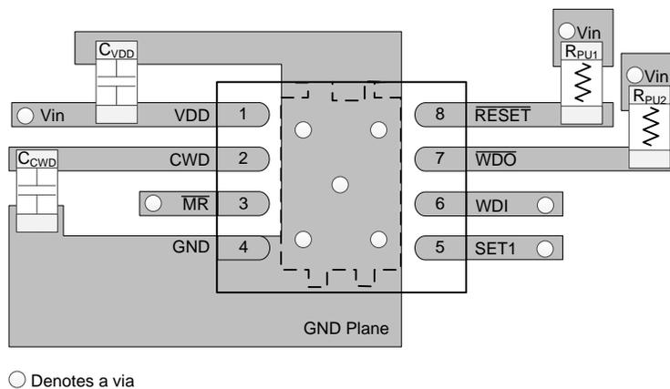
**Figure 26. Typical Layout For TPS3852**
