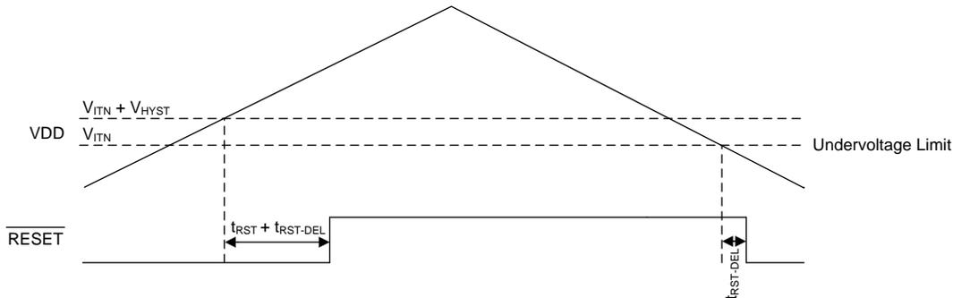
**Figure 16. Undervoltage Detection**
