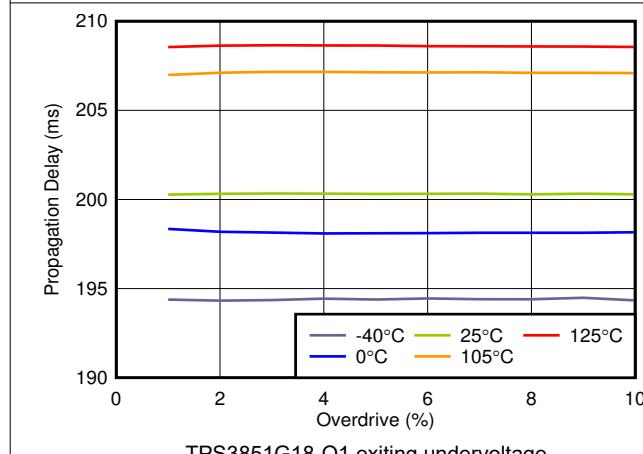
图 6-17. Propagation Delay ( $t_{RST}$ ) vs Overdrive
