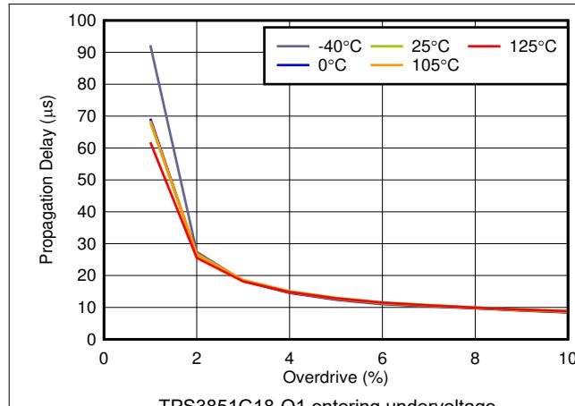
图 6-15. Propagation Delay vs Overdrive
