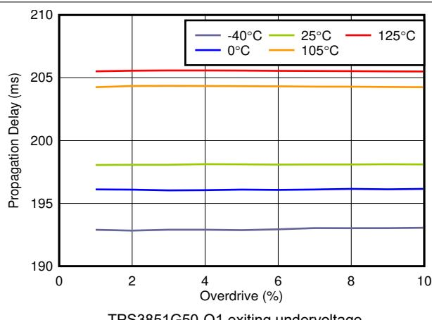
图 6-18. Propagation Delay ( $t_{RST}$ ) vs Overdrive
