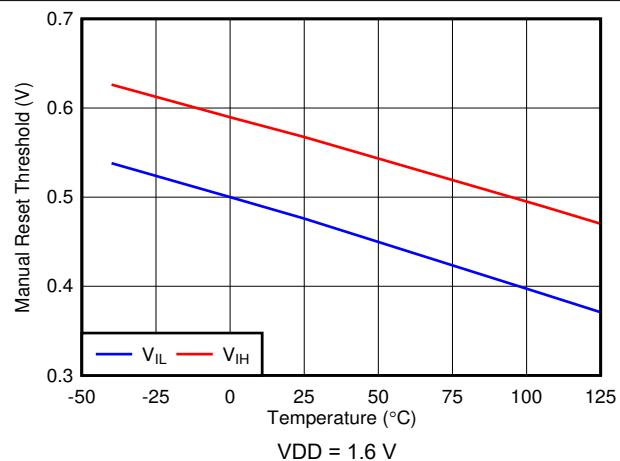
图 6-4. MR Threshold vs Temperature
