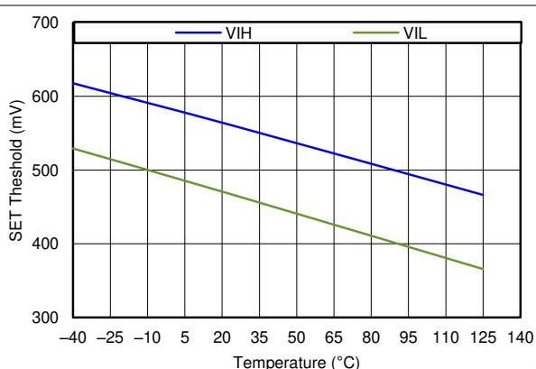
図 5-14. SET Threshold vs Temperature
