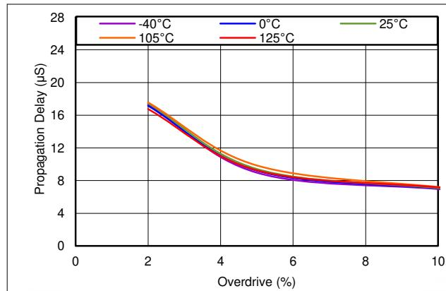
图 5-8. Undervoltage Propagation Delay vs Overdrive
