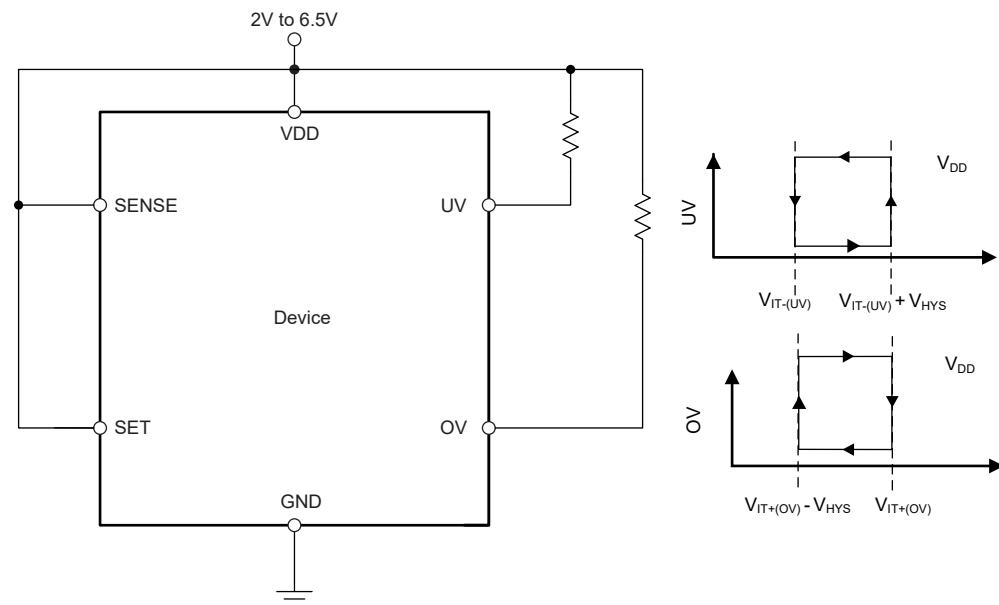
図 7-4. Monitoring the Same Voltage as  $V_{DD}$  with Wired-OR Logic
