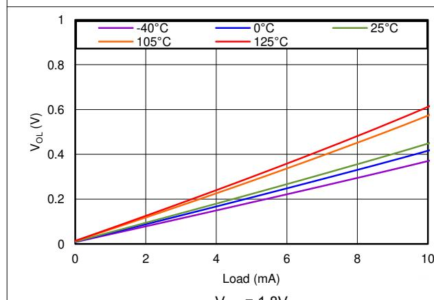
图 5-12. Low-Level Output Voltage vs Output Current
