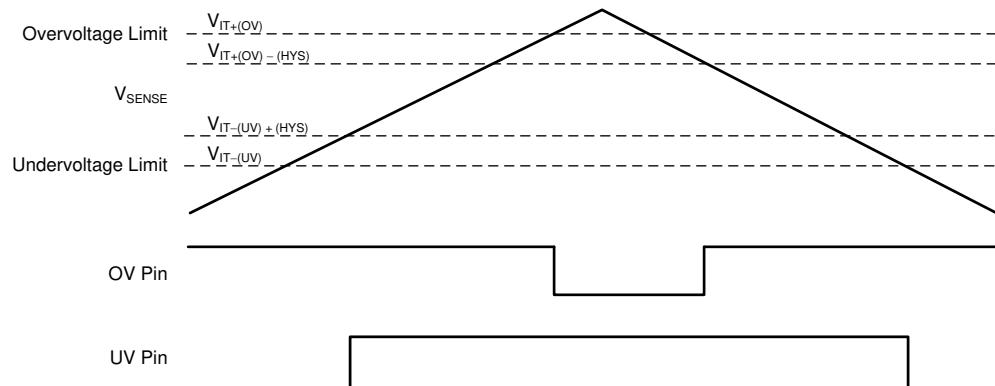
図 7-1. Window Voltage Detector Operation
