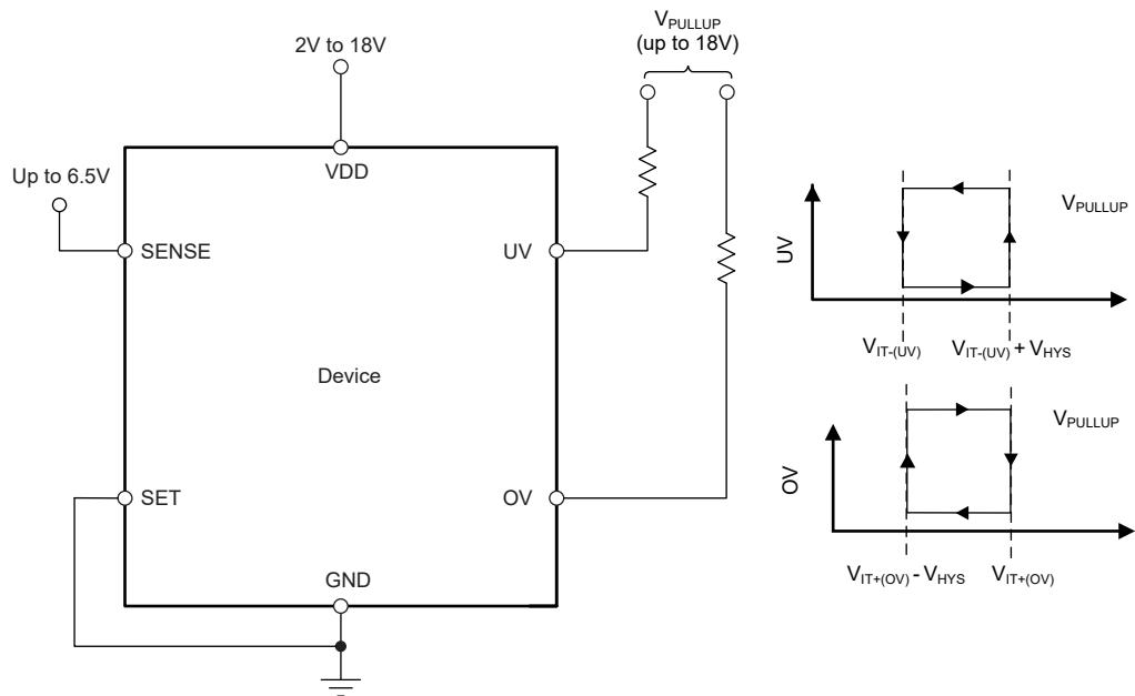
図 7-3. Interfacing to Voltages Other Than  $V_{DD}$
