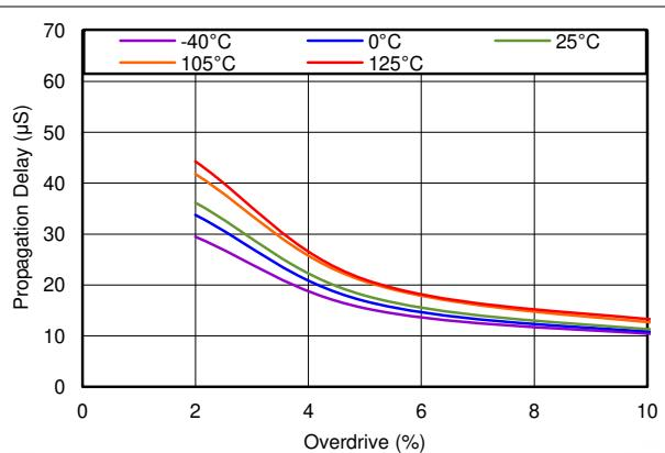
图 5-9. Ovvervoltage Propagation Delay vs Overdrive
