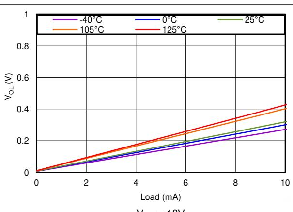
图 5-13. Low-Level Output Voltage vs Output Current
