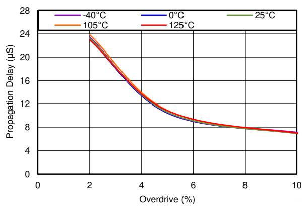
图 5-11. Ovvervoltage Propagation Delay vs Overdrive
