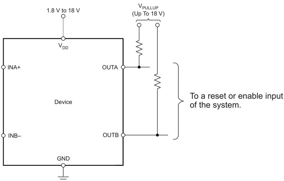
Figure 16. Interfacing to Voltages Other Than  $V_{DD}$
