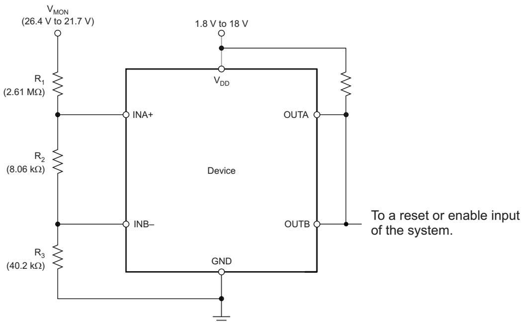
NOTE: The inputs can monitor a voltage higher than  $V_{DDmax}$  with the use of an external resistor divider network.
