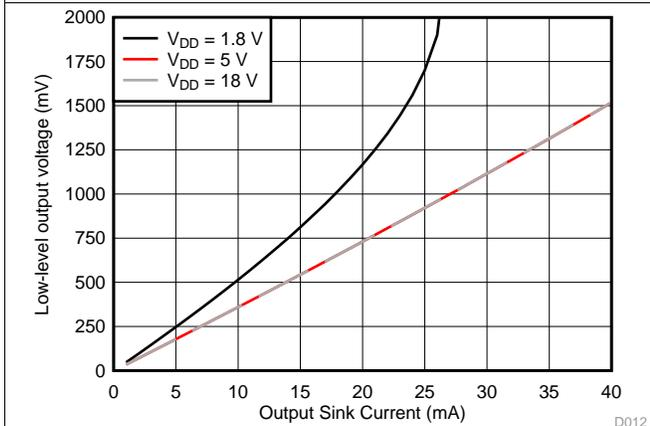
Figure 12. Output Voltage Low ( $V_{OL}$ ) vs Output Sink Current ( $85^\circ\text{C}$ )
