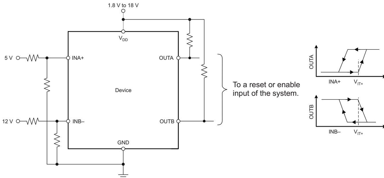
NOTE: In this case, OUTA is driven low when an undervoltage condition is detected at the 5-V rail and OUTB is driven low when an overvoltage condition is detected at the 12-V rail.
