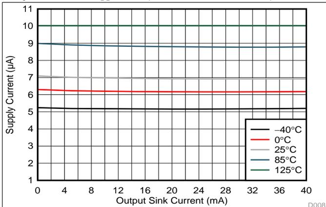
Figure 8. Supply Current ( $I_{DD}$ ) vs Output Sink Current
