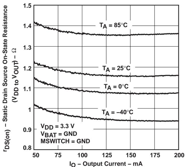
**STATIC DRAIN SOURCE ON-STATE RESISTANCE
