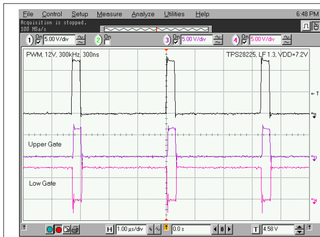
Fig 7-4. 12-V PWM Pulse at V_{DD} = 7.2\text{ V}
