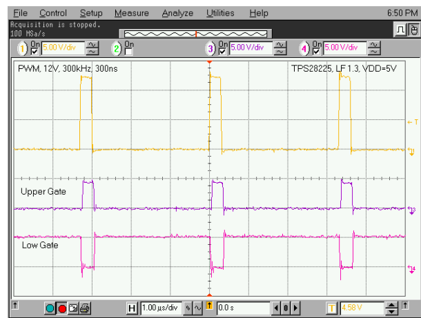
Figure 6-5. 12-V PWM Pulse at V_{DD} = 5\text{ V}
