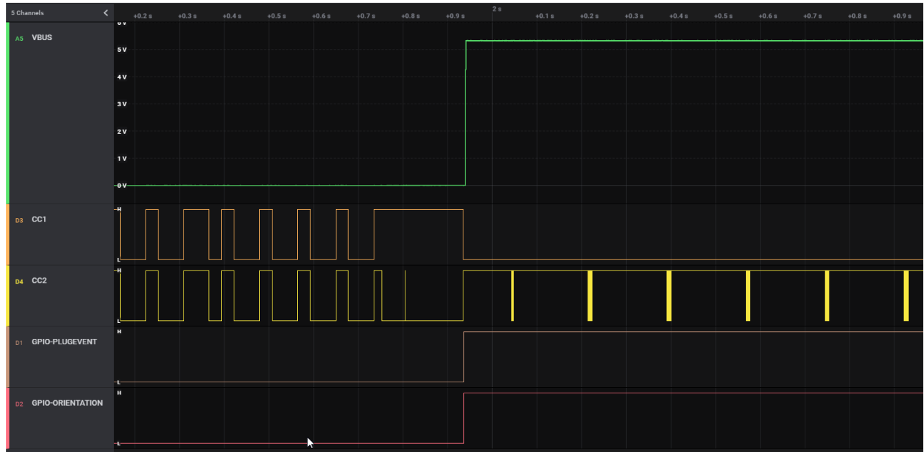
図 8-21. USB SuperSpeed Mux Control - Flipped Orientation
