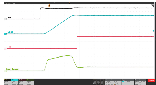
9-6. Start-up with EN/UVLO: V_{IN} = 12 V, EN/UVLO Stepped Up From 0 V to 3 V, C_{LOAD} = 50 mF, R_{LOAD(Start-up)} = 0.48 \Omega , C_{DVRT} = 33 nF, V_{IREF} = 1 V, R_{ILIM(TPS25990)} = 422 \Omega , and R_{ILIM(TPS25985)} = 316 \Omega
