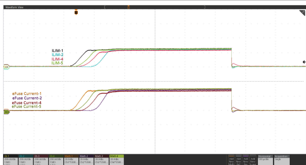
Figure 9-8. Power Up into Short (Current distribution among five devices in parallel): V_{IN} = 12 V, EN/UVLO Stepped Up From 0 V to 3 V, R_{REF} = 40.2 k \Omega , R_{LIM} on Each Device = 300 \Omega , and OUT Shorted to GND
