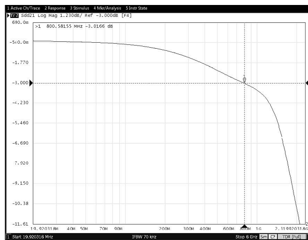
8-23. Data Transmission Characteristics vs Frequency
