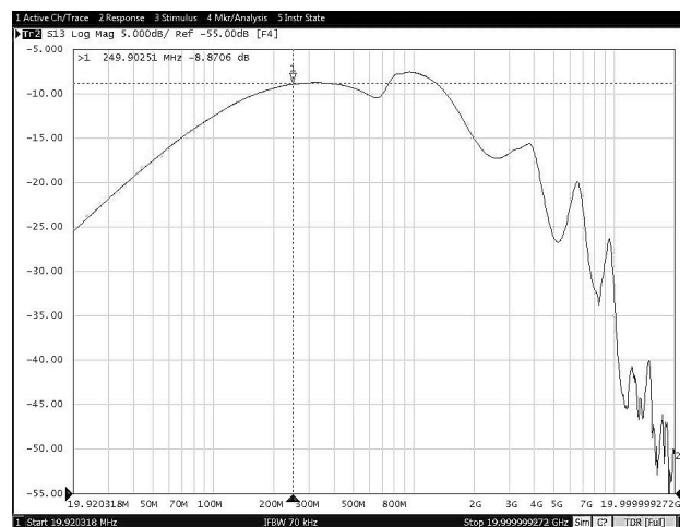
8-24. Off-state Data-Switch Isolation vs Frequency
