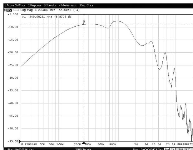
8-32. Off-State Data-Switch Isolation vs Frequency (TPS25830-Q1)
