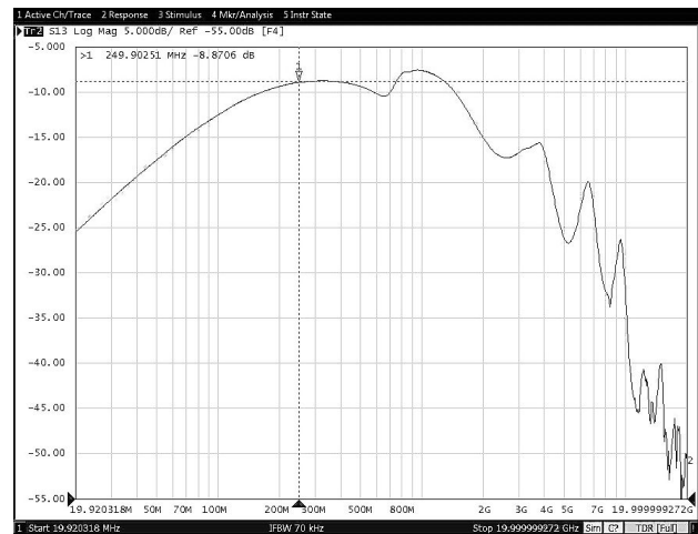
8-30. Off-State Data-Switch Isolation vs Frequency (TPS25830A-Q1)
