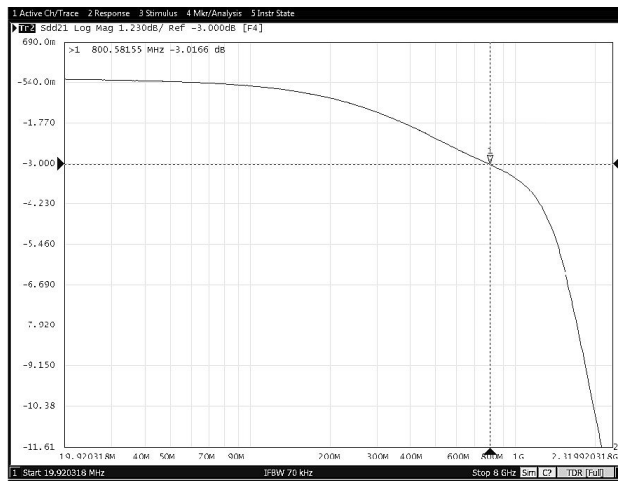
8-29. Data Transmission Characteristics vs Frequency (TPS25830A-Q1)
