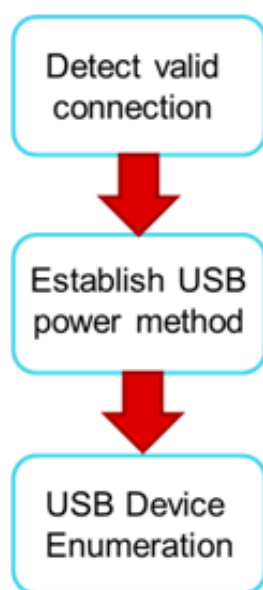
Figure 11. Flow of DFP to UFP Configuration
