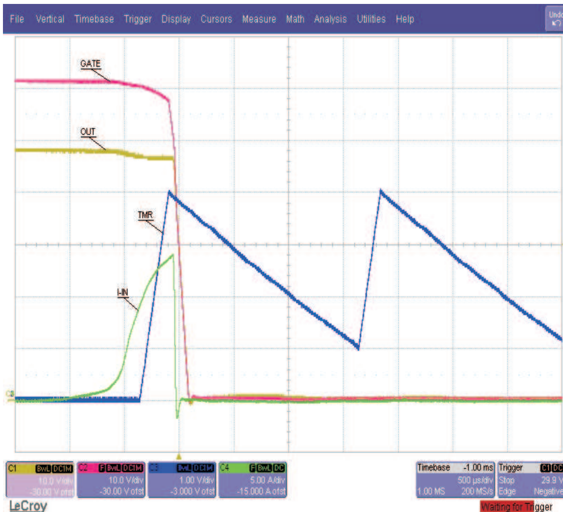
Figure 16. TPS2480/81 Restart Cycle Timing
