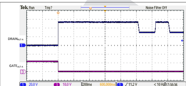
图 10-4. Backoff due to PCut Fault
