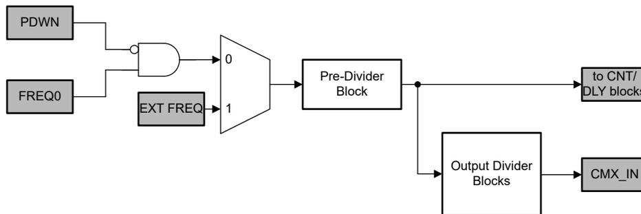
**Figure 8-49. Fixed frequency oscillator block diagram**
