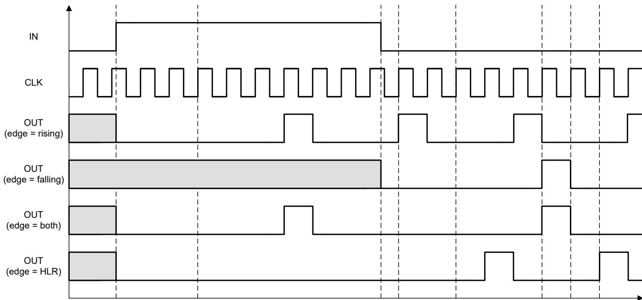
**Figure 7-16. Counter Output Timing Example (DATA = 3)**
