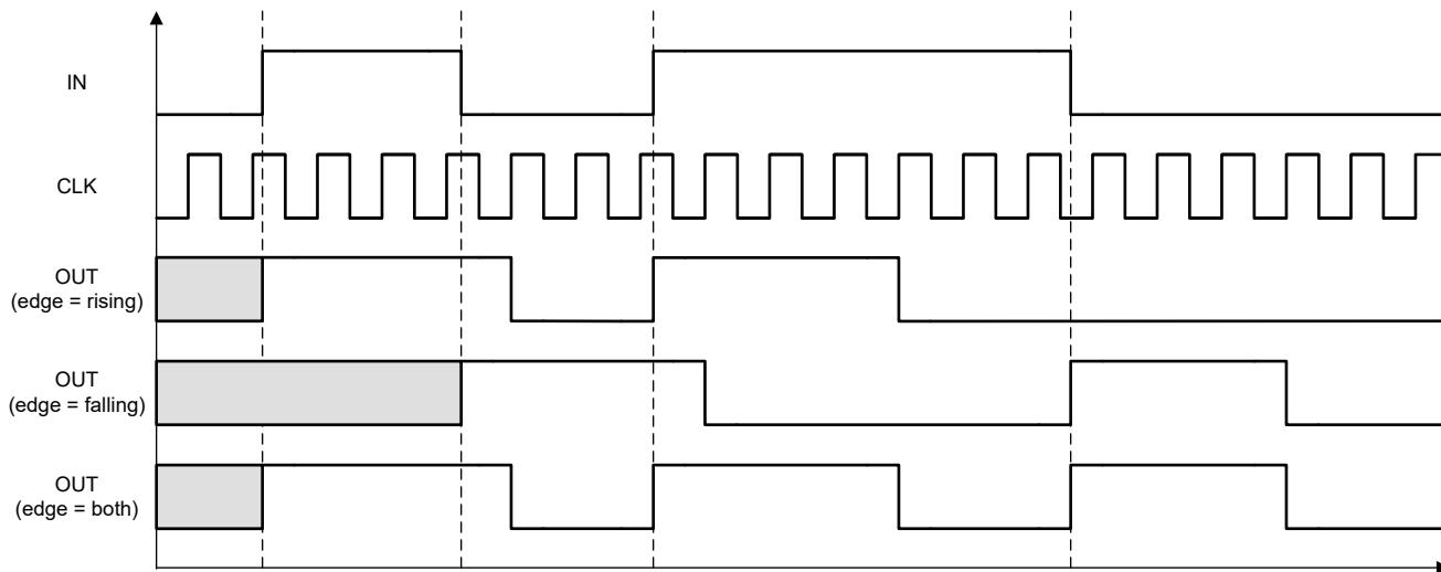
Figure 7-18. One-shot output timing example (DATA = 2)
