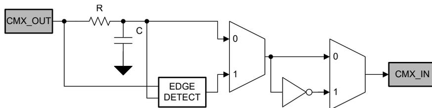
**Figure 8-24. Deglitch Filter or Edge Detector Block Diagram**
