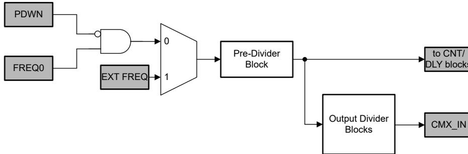
**Figure 8-48. Fixed frequency oscillator block diagram**
