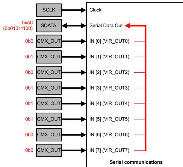
Figure 8-63. Serial Communications for Parallel-to-Serial Block Diagram
