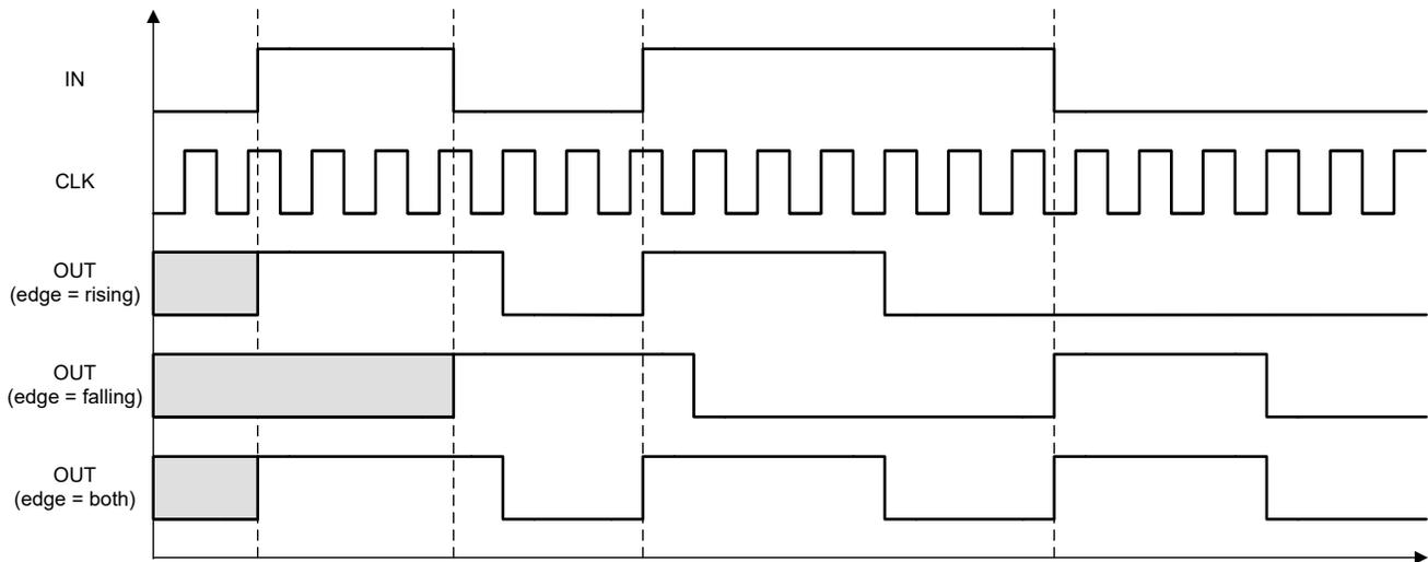
Figure 8-18. One-shot output timing example (DATA = 2)
