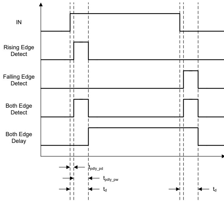
**Figure 7-23. Delayed edge detector output timing diagram**
