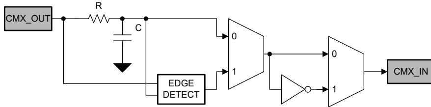
**Figure 7-24. Deglitch Filter or Edge Detector Block Diagram**
