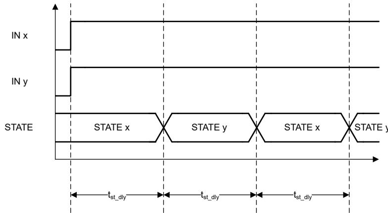
**Figure 7-34. Closed loop state transition timing example**
