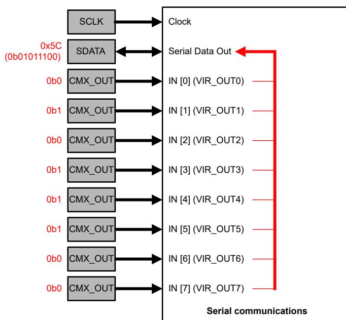
Figure 7-63. Serial Communications for Parallel-to-Serial Block Diagram
