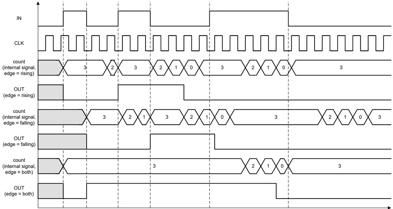
**Figure 8-19. Frequency detector output timing example (DATA = 3)**
