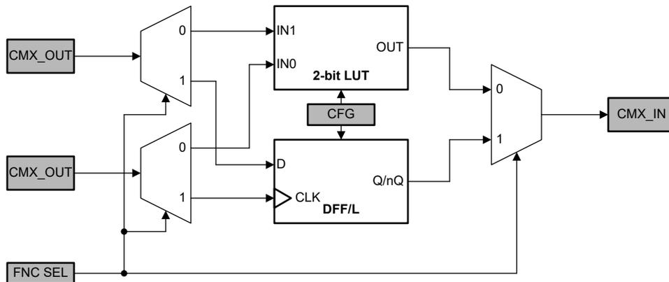
**Figure 8-2. 2-bit LUT or DFF/Latch Block Diagram**
