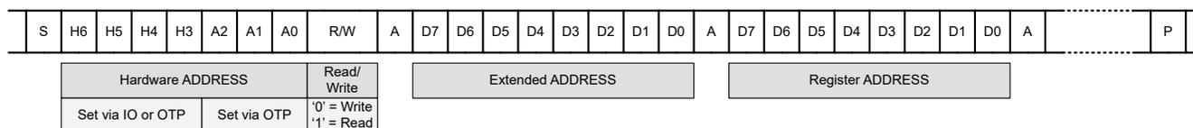
**Figure 8-52. TPLD I<sup>2</sup>C Frame and Formatting**
