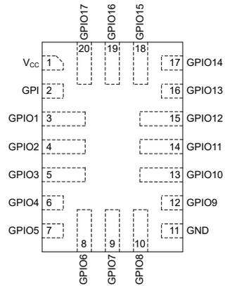
**Figure 4-2. RJY Package, 20-pin UQFN (top view)**
