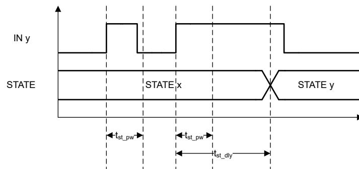
**Figure 7-27. State transition trigger requirements timing example**
