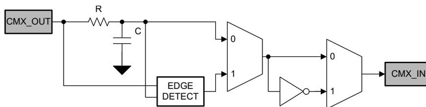
**Figure 8-24. Deglitch Filter or Edge Detector Block Diagram**
