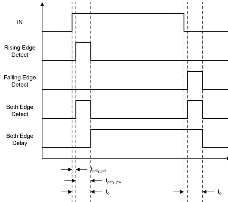
**Figure 8-23. Delayed edge detector output timing diagram**
