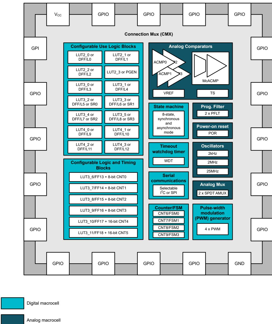
Figure 7-1. TPLD2001 Functional Block Diagram
