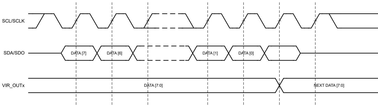
Figure 7-64. Serial Communications for Parallel-to-Serial Timing Example
