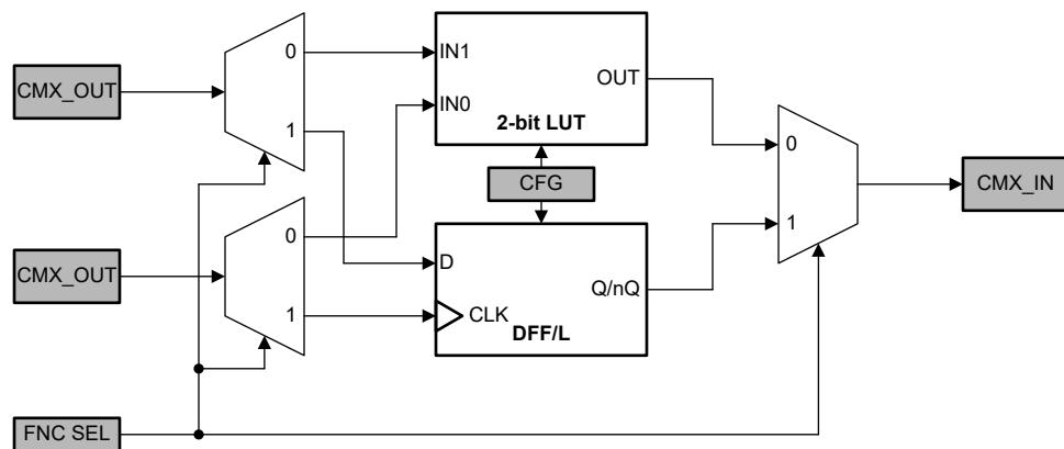
**Figure 7-2. 2-bit LUT or DFF/Latch Block Diagram**
