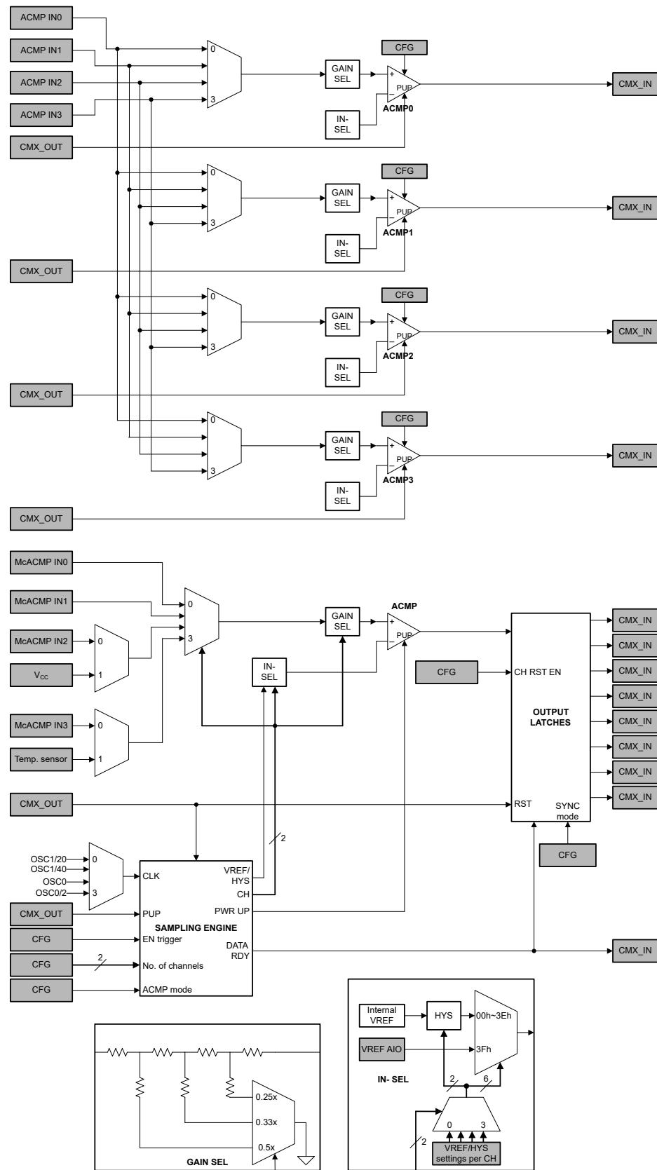
Figure 7-43. Analog Comparators Block Diagram
