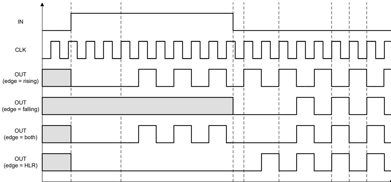
**Figure 7-15. Counter Output Timing Example (DATA = 1)**
