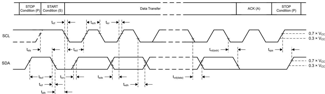
**Figure 8-51. I<sup>2</sup>C Read/Write Timing Diagram**
