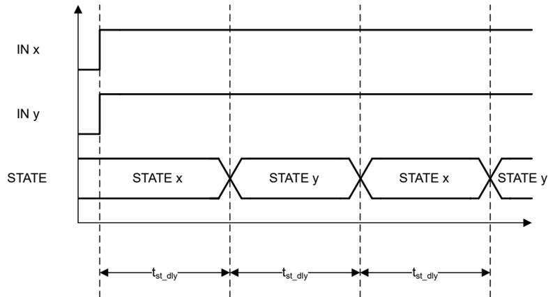
**Figure 8-34. Closed loop state transition timing example**
