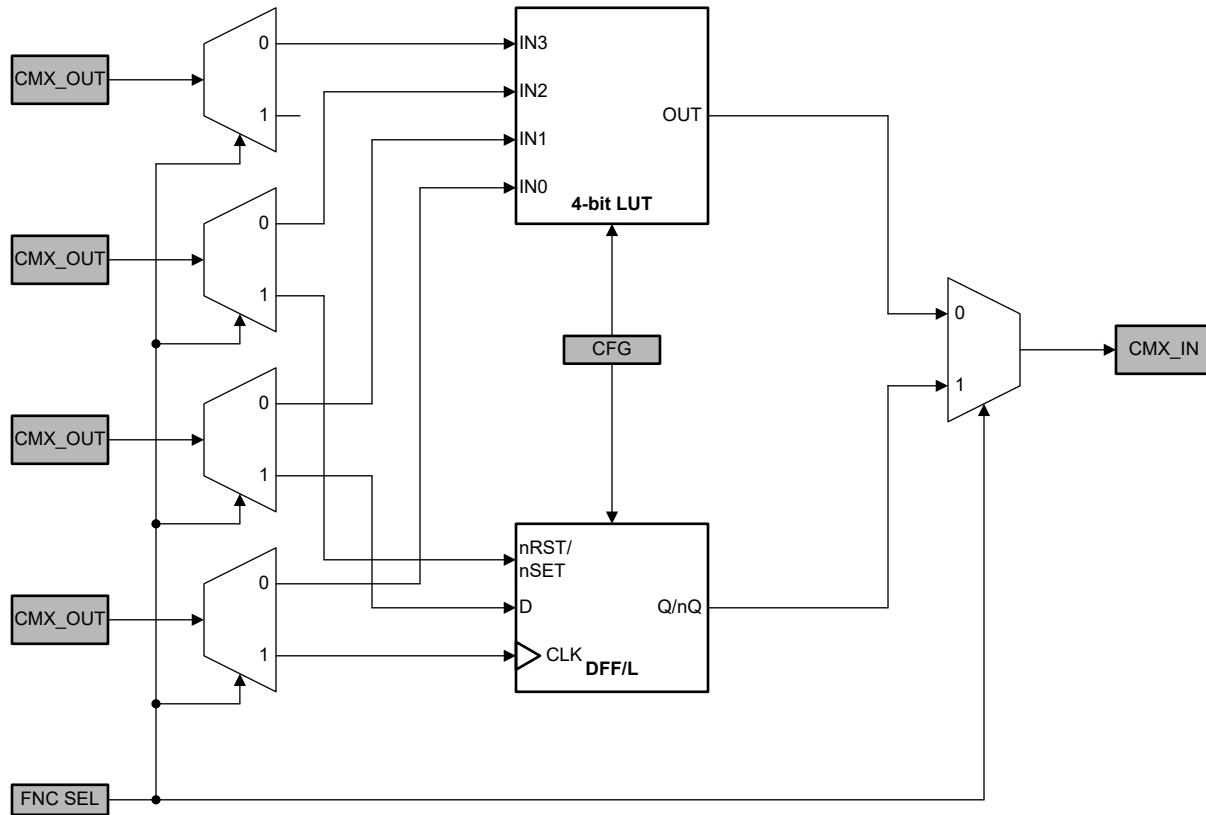
Figure 7-11. 4-bit LUT or DFF/Latch Block Diagram
