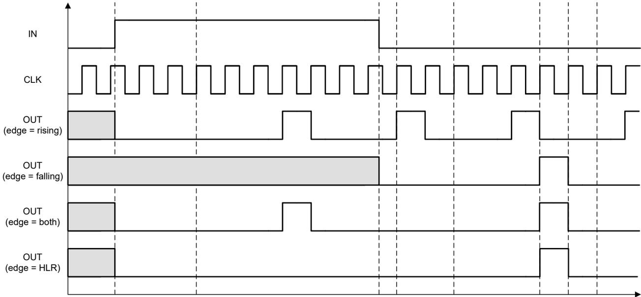
Figure 8-16. Counter Output Timing Example (DATA = 3)
