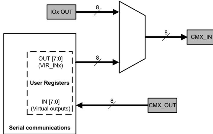
**Figure 8-60. Serial Communications Block Diagram**
