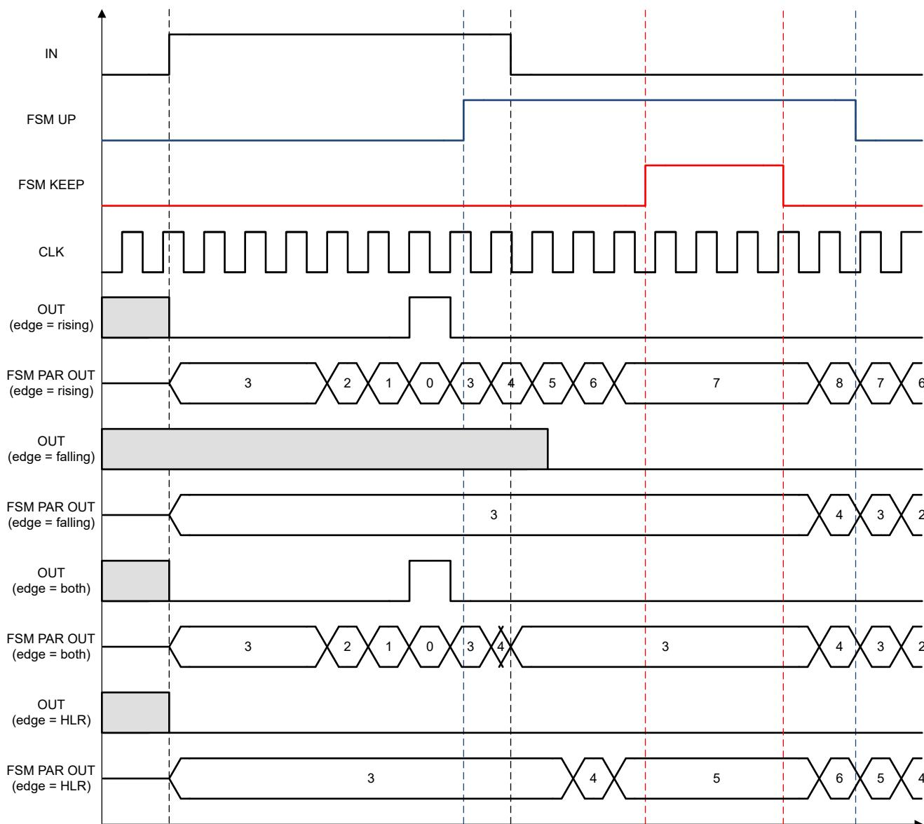
**Figure 7-37. CNT/FSM with UP/KEEP timing example (DATA = 3)**
