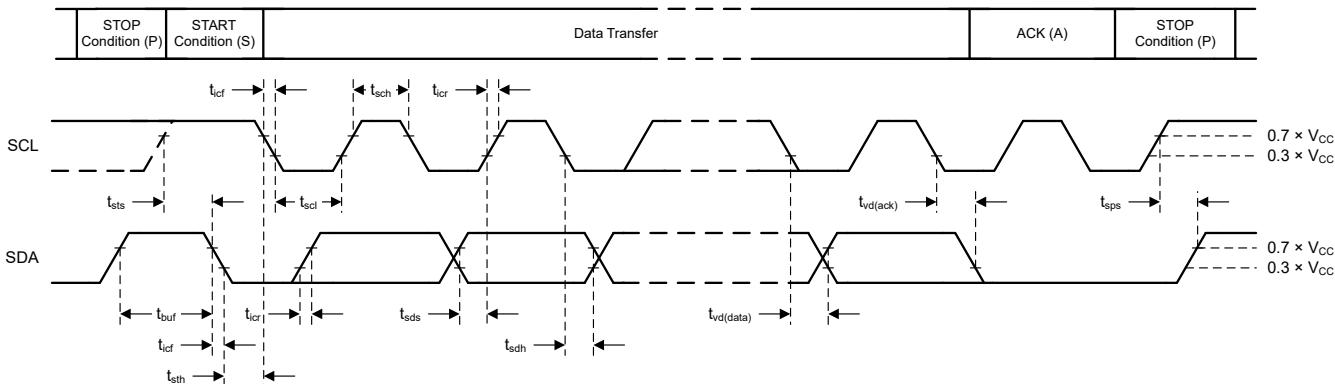
**Figure 7-51. I<sup>2</sup>C Read/Write Timing Diagram**
