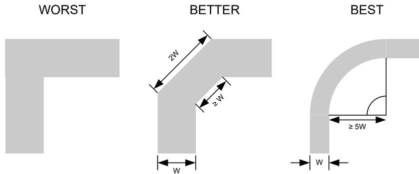
**Figure 9-3. Example trace corners for improved signal integrity**
