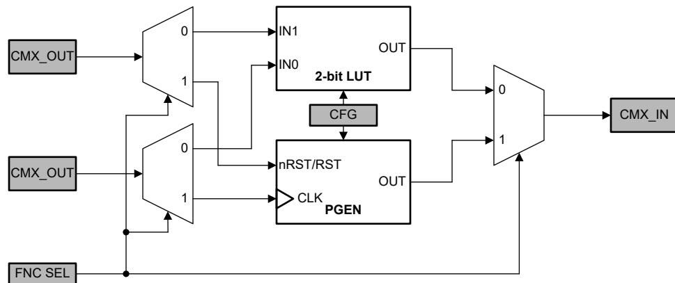
**Figure 7-3. 2-bit LUT or Pattern Generator Block Diagram**
