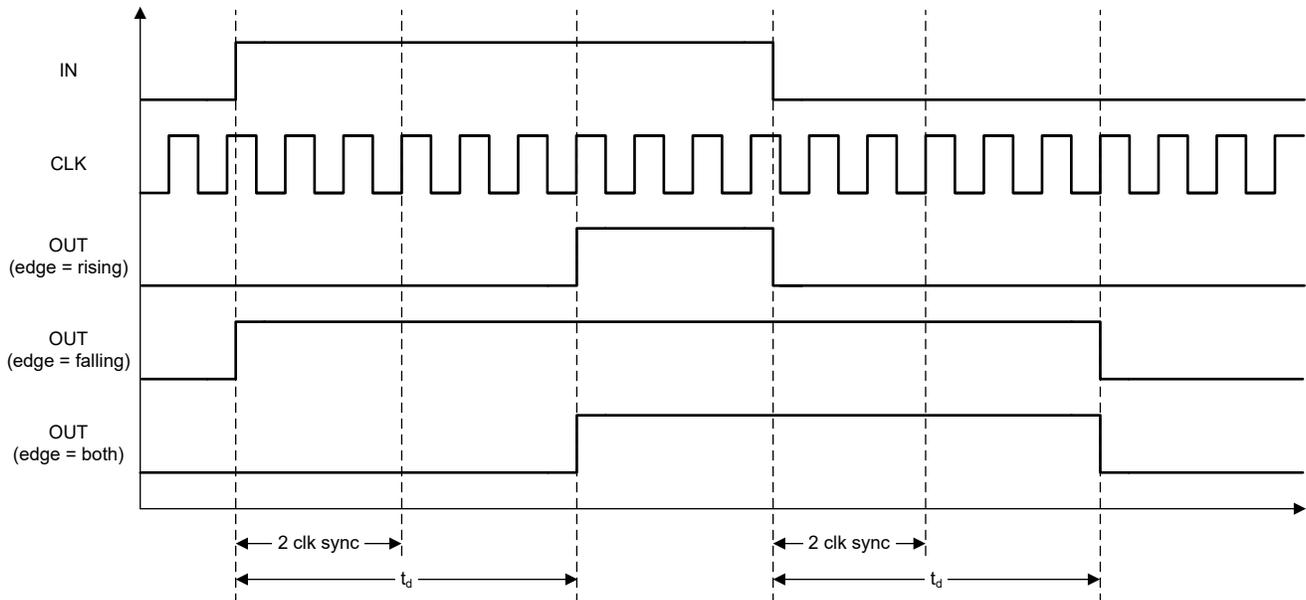
**Figure 8-14. Delay Output Timing Example (DATA = 3)**
