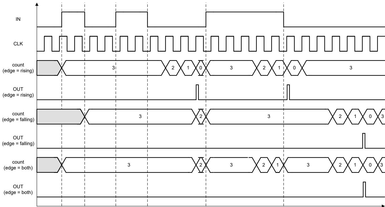
Figure 7-21. Delayed edge detector output timing example (DATA = 3)
