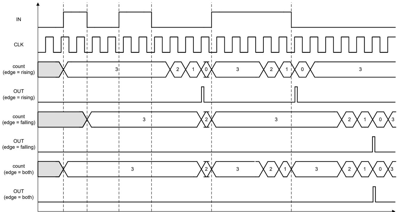
**Figure 8-21. Delayed Edge Detector Output Timing Example (DATA = 3)**
