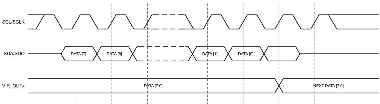
**Figure 8-64. Serial Communications for Parallel-to-Serial Timing Example**
