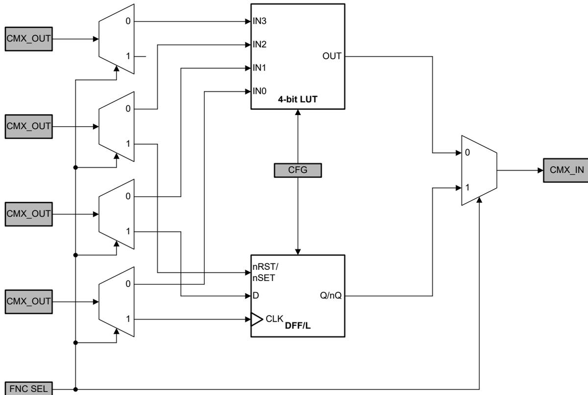
**Figure 8-11. 4-bit LUT or DFF/Latch Block Diagram**
