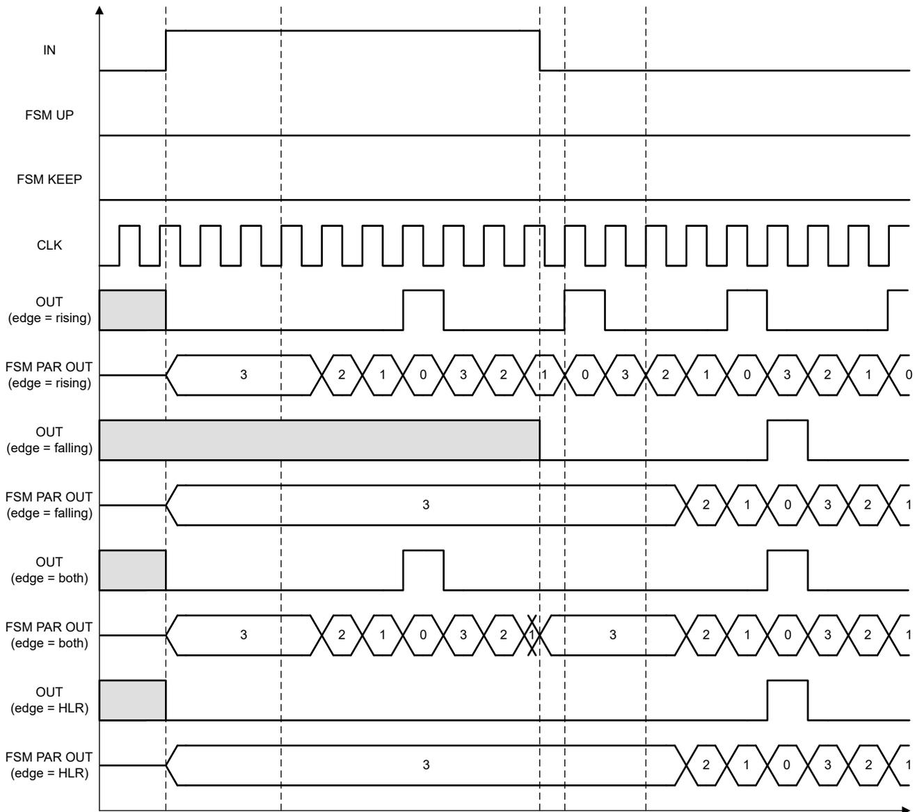
**Figure 8-36. CNT/FSM timing example (DATA = 3)**
