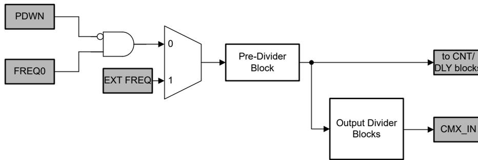
Figure 8-47. Fixed frequency oscillator block diagram
