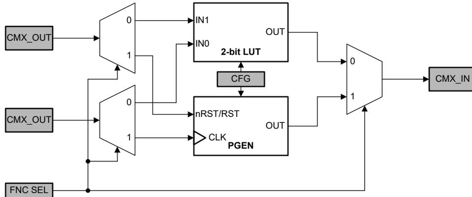
Figure 8-3. 2-bit LUT or Pattern Generator Block Diagram
