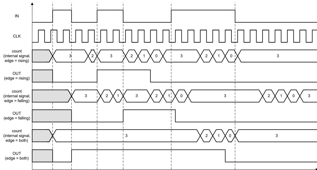
**Figure 7-19. Frequency comparator output timing example (DATA = 3)**
