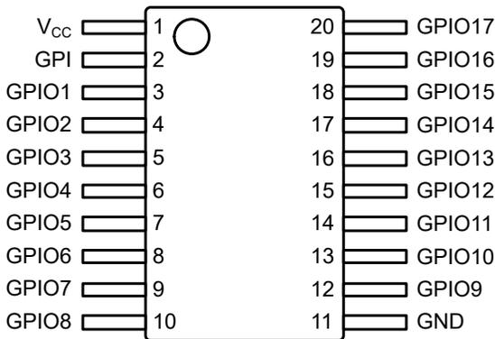
**Figure 4-1. DGS Package, 20-Pin VSSOP (top view)**
