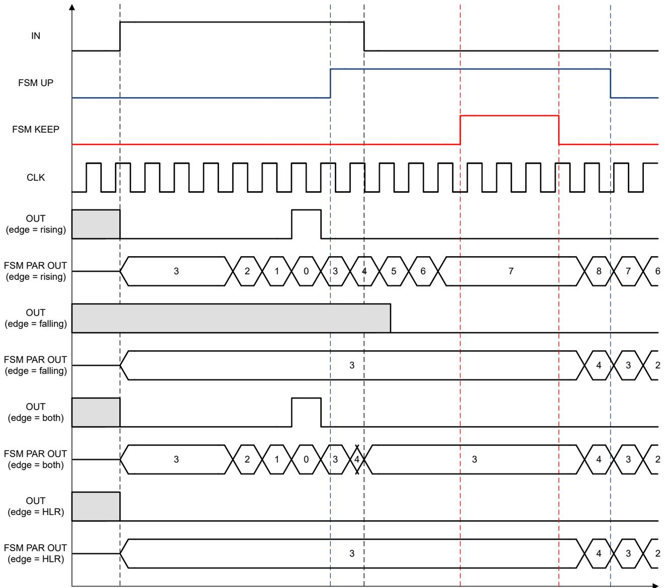
Figure 8-37. CNT/FSM with UP/KEEP timing example (DATA = 3)
