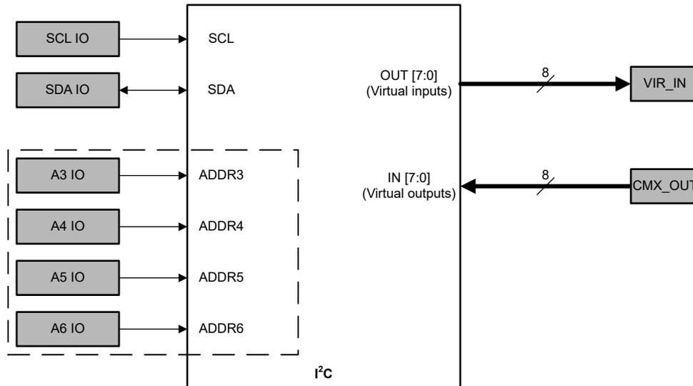
**Figure 8-50. I<sup>2</sup>C Serial Communications GPIO Allocation**
