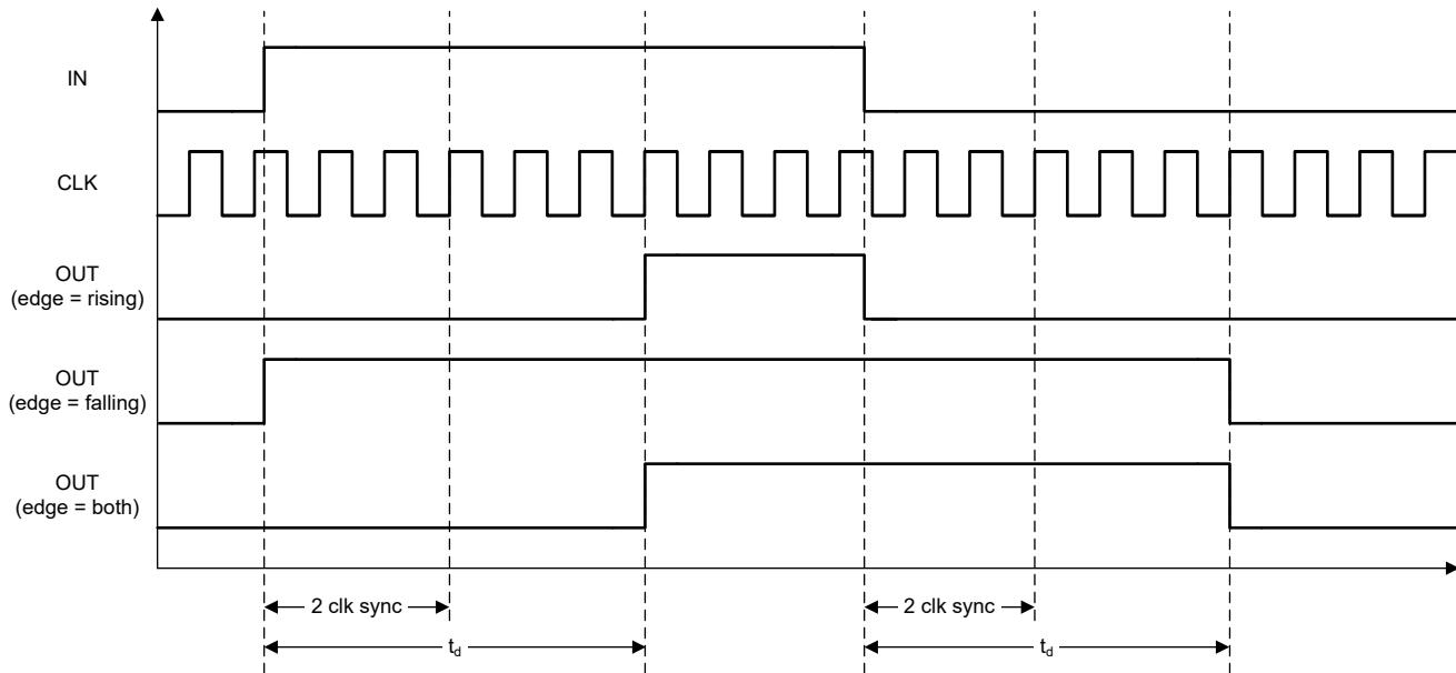
Figure 7-14. Delay Output Timing Example (DATA = 3)
