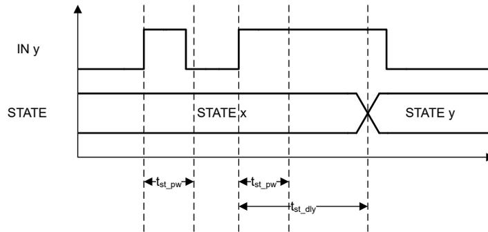
**Figure 8-27. State transition trigger requirements timing example**
