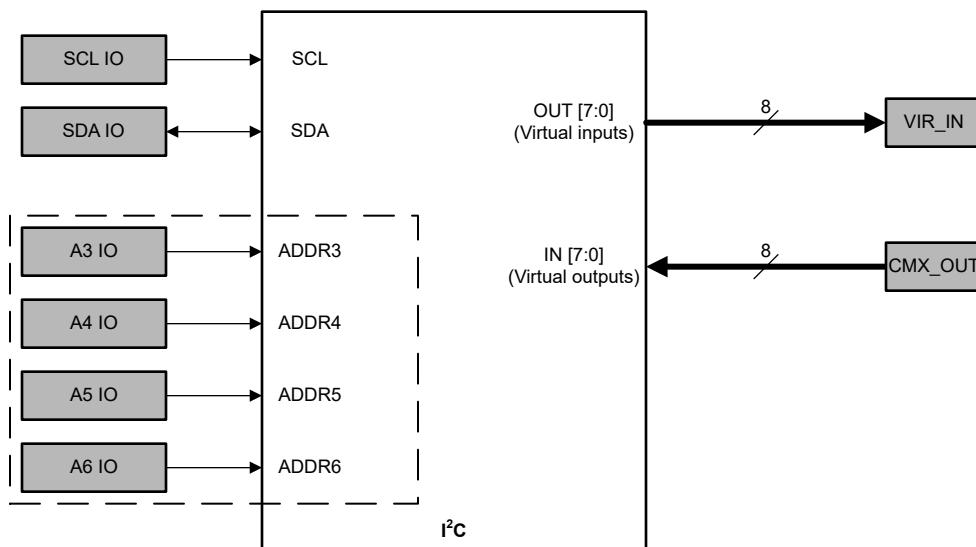
**Figure 7-50. I<sup>2</sup>C Serial Communications GPIO Allocation**
