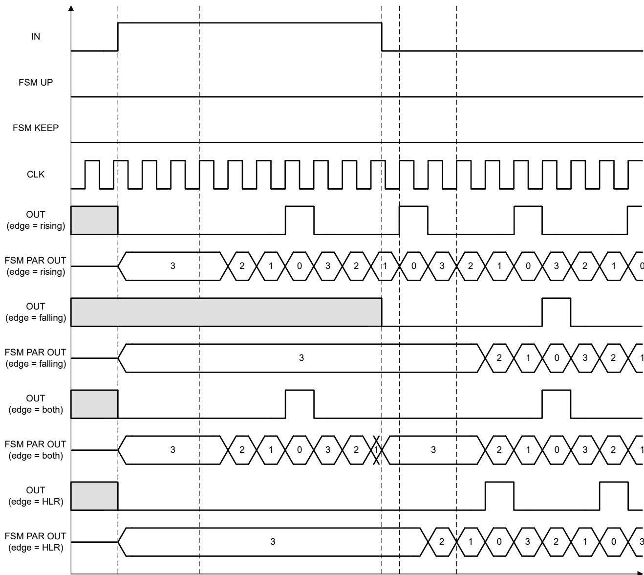
Figure 7-36. CNT/FSM timing example (DATA = 3)
