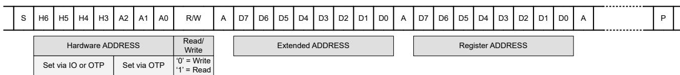
**Figure 7-52. TPLD I<sup>2</sup>C Frame and Formatting**
