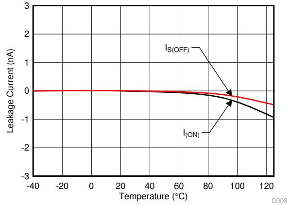
図 5-8. Leakage Current vs Temperature
