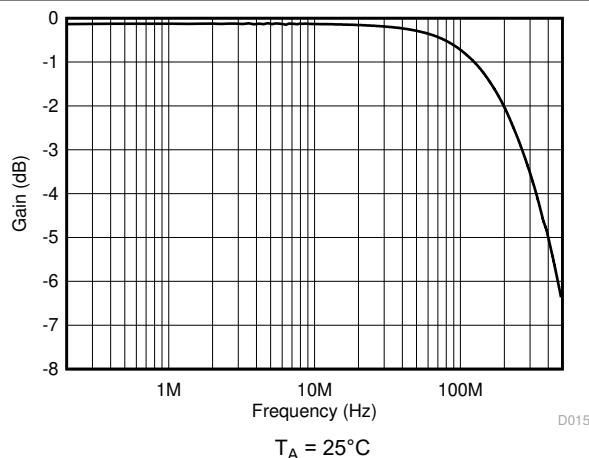
図 5-15. On Response vs Frequency
