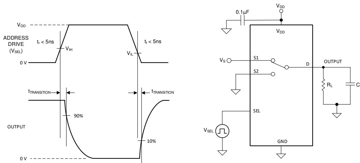
**図 6-4. Transition-Time Measurement Setup**
