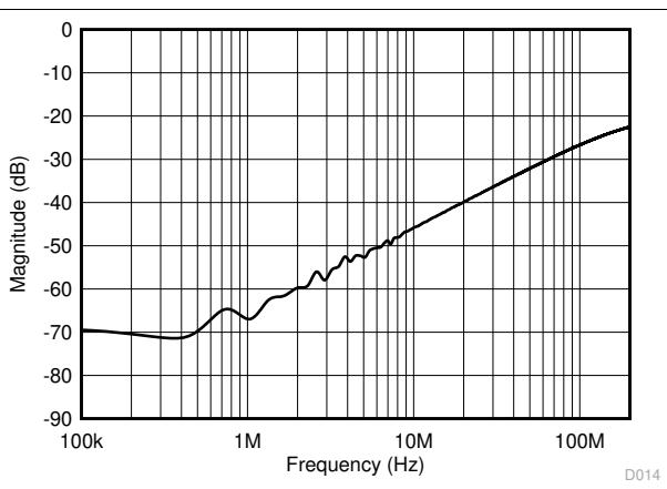
図 5-14. Xtalk and Off-Isolation vs Frequency
