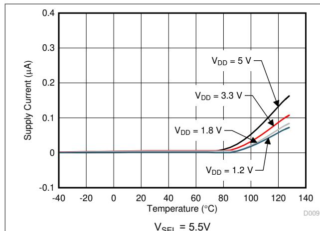
図 5-9. Supply Current vs Temperature
