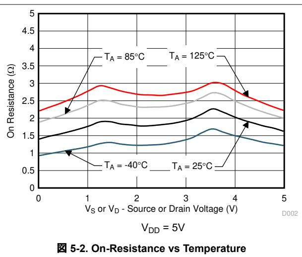
図 5-2. On-Resistance vs Temperature
