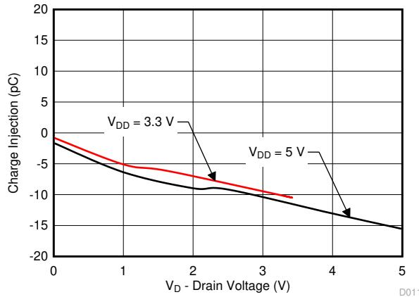
[図 7-4. Charge Injection vs Drain Voltage](#)
