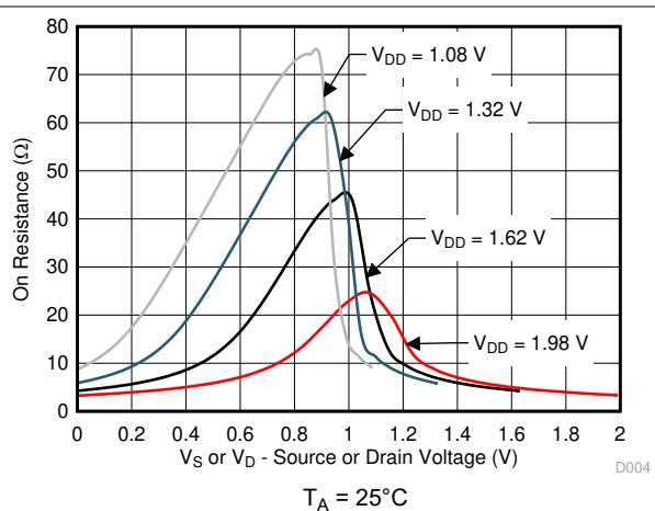
図 5-4. On-Resistance vs Source or Drain Voltage
