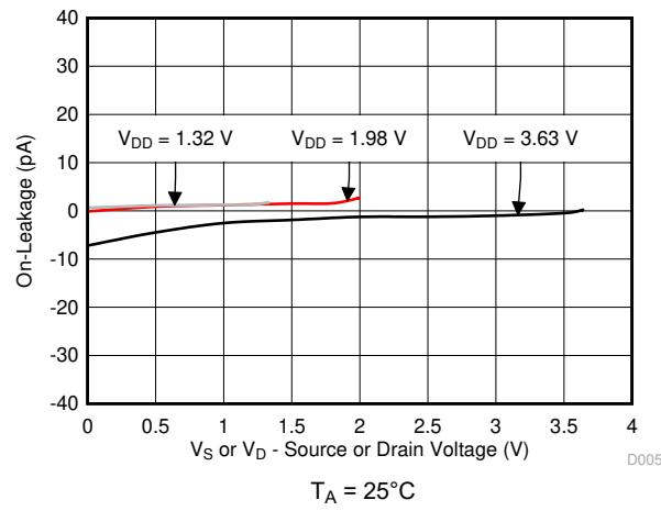
図 5-5. On-Leakage vs Source or Drain Voltage
