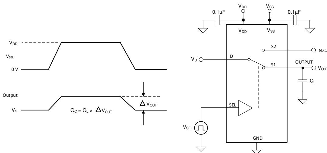
**図 6-6. Charge-Injection Measurement Setup**
