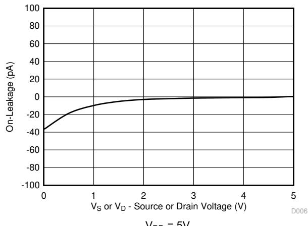
図 5-6. On-Leakage vs Source or Drain Voltage
