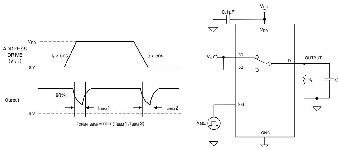
**図 6-5. Break-Before-Make Delay Measurement Setup**
