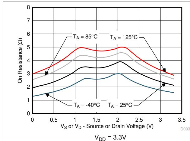
図 5-3. On-Resistance vs Temperature
