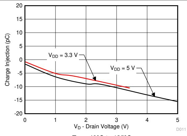
図 5-11. Charge Injection vs Drain Voltage
