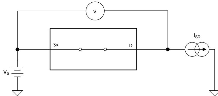
**図 6-1. On-Resistance Measurement Setup**
