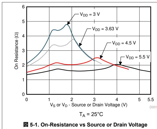
図 5-1. On-Resistance vs Source or Drain Voltage
