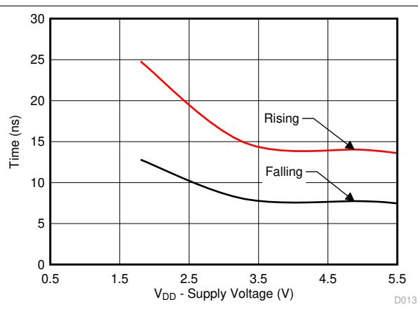
図 5-13. Output  $T_{\text{TRANSITION}}$  vs Supply Voltage
