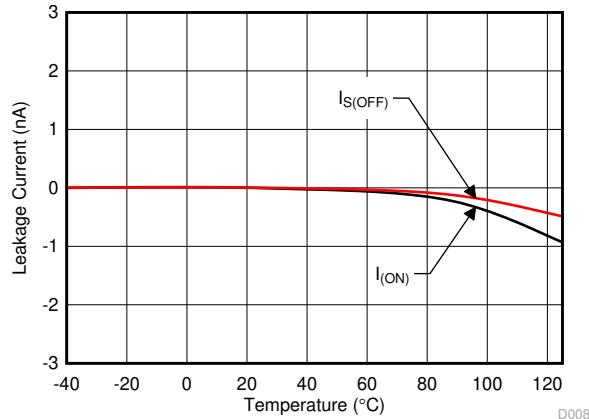
図 7-2. Leakage Current vs Temperature
