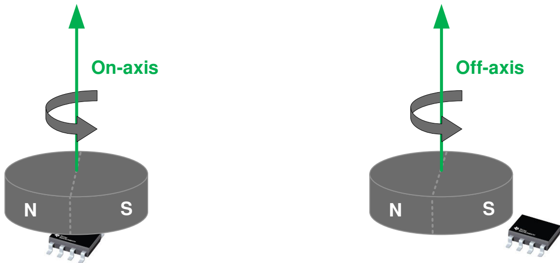
图 8-5. On-Axis vs. Off-Axis Angle Measurements
