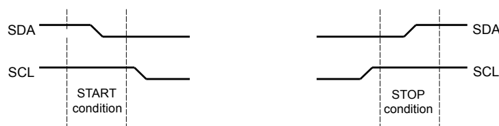
Figure 18-3. START and STOP Conditions
