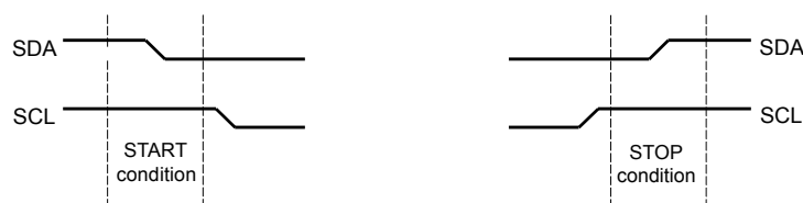
Figure 18-3. START and STOP Conditions
