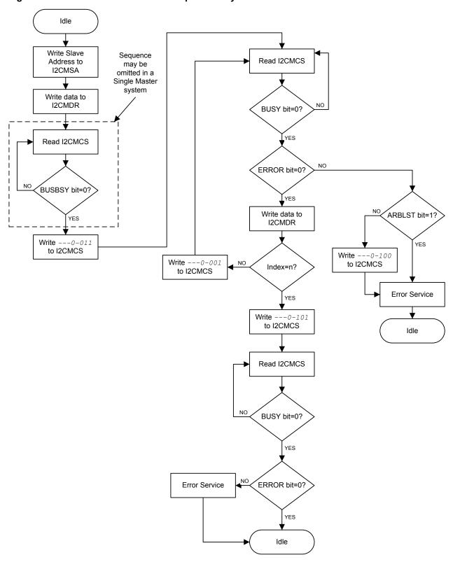
Figure 15-10. Master TRANSMIT of Multiple Data Bytes
