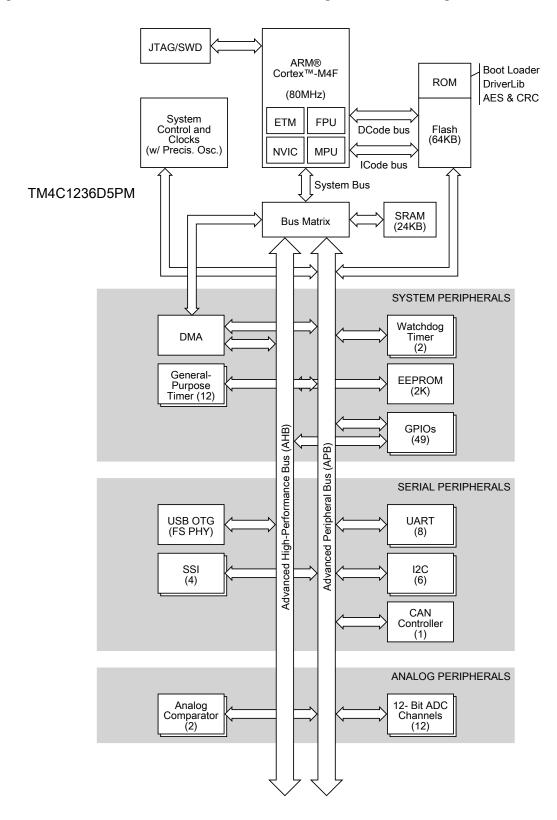
Figure 1-1. Tiva<sup>™</sup> TM4C1236D5PM Microcontroller High-Level Block Diagram
