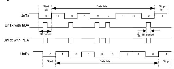
Figure 13-3. IrDA Data Modulation
