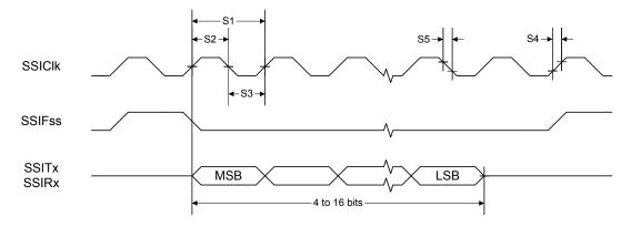
Figure 21-19. SSI Timing for MICROWIRE Frame Format (FRF=10), Single Transfer
