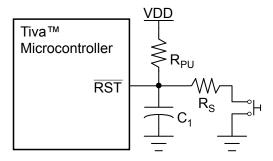
Typical  $R_{PU} = 10 \text{ k}\Omega$
