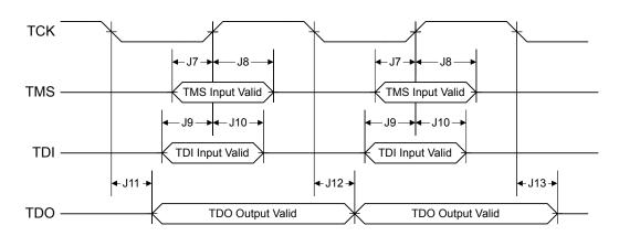
Figure 21-3. JTAG Test Access Port (TAP) Timing
