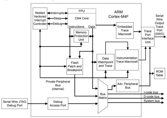
Figure 2-1. CPU Block Diagram
