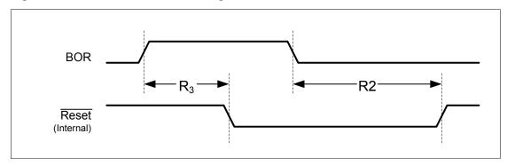
Figure 21-11. External Reset Timing (RST)
