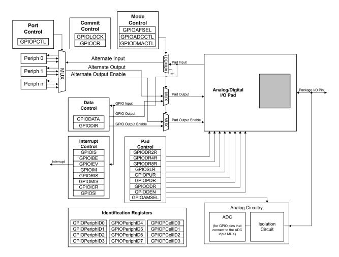
Figure 9-2. Analog/Digital I/O Pads
