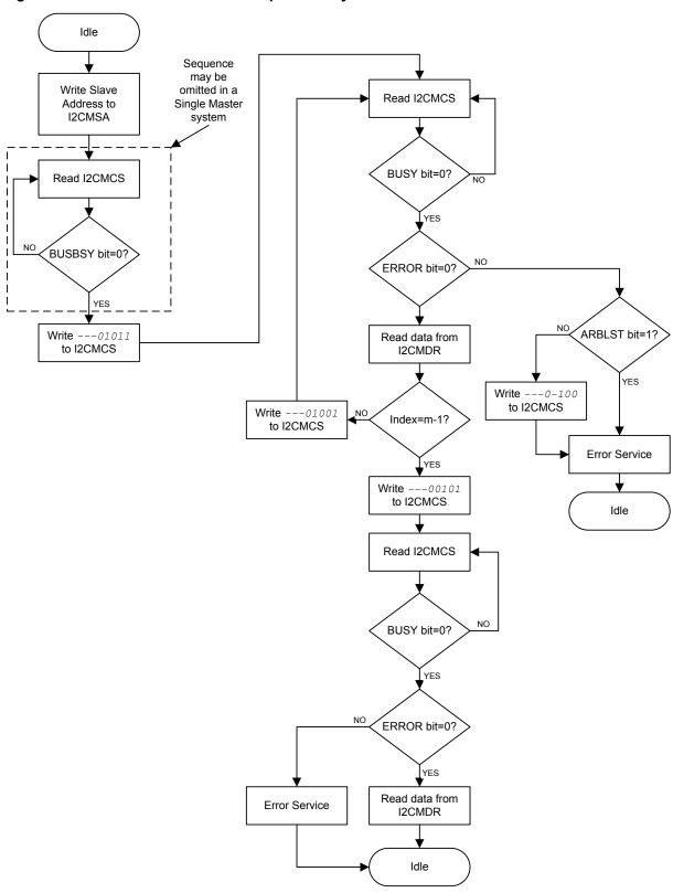
Figure 15-11. Master RECEIVE of Multiple Data Bytes
