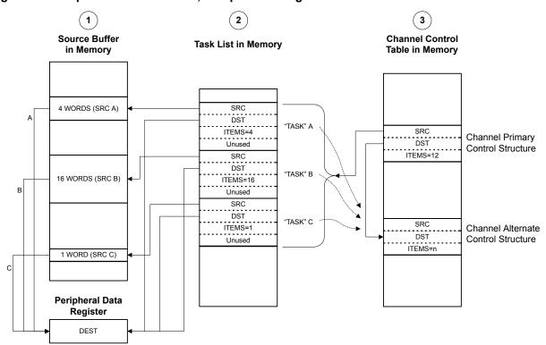
Figure 8-5. Peripheral Scatter-Gather, Setup and Configuration
