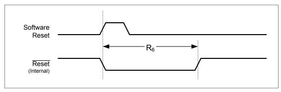
Figure 21-13. Watchdog Reset Timing
