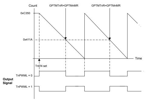
Figure 10-5. 16-Bit PWM Mode Example
