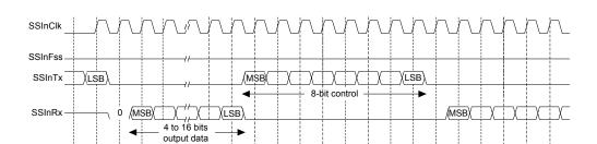
Figure 14-11. MICROWIRE Frame Format (Continuous Transfer)
