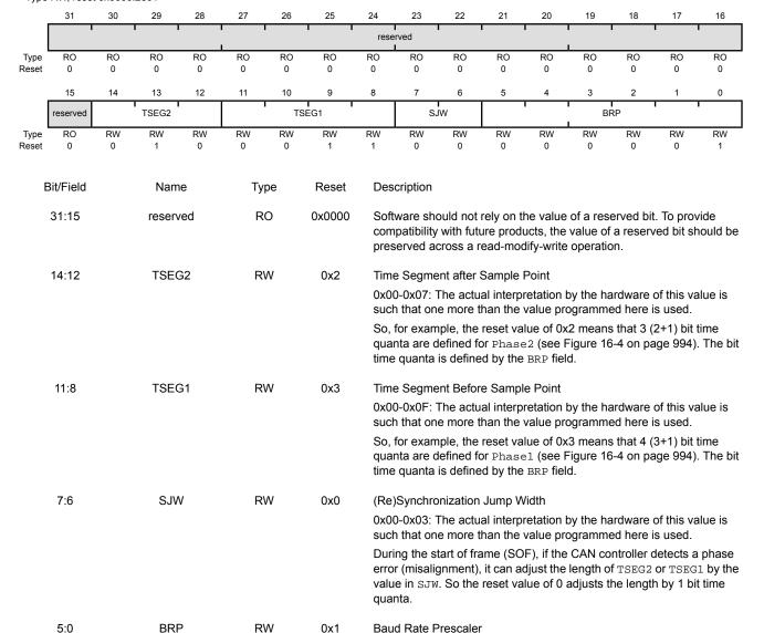
The value by which the oscillator frequency is divided for generating the bit time quanta. The bit time is built up from a multiple of this quantum. 0x00-0x03F: The actual interpretation by the hardware of this value is such that one more than the value programmed here is used. BRP defines the number of CAN clock periods that make up 1 bit time
