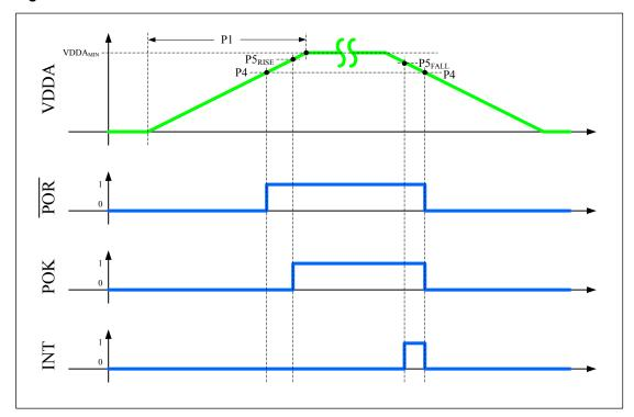
Figure 21-4. Power Assertions versus VDDA Levels
