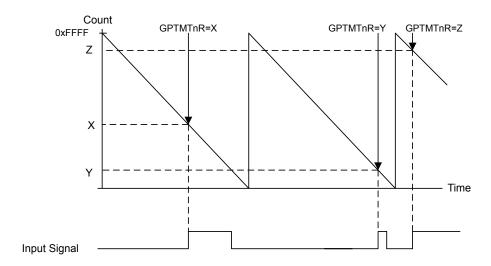
Figure 10-4. 16-Bit Input Edge-Time Mode Example
