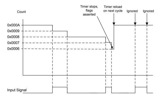
Figure 10-3. Input Edge-Count Mode Example, Counting Down
