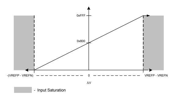
Figure 12-10. Differential Voltage Representation
