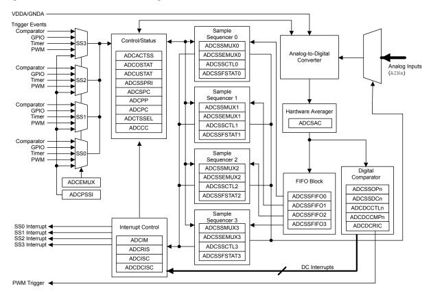
Figure 12-2. ADC Module Block Diagram
