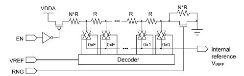
**Note:** In the figure above, N\*R represents a multiple of the R value that produces the results specified in Table 18-2 on page 1148.
