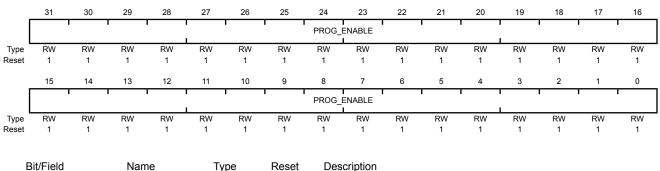
31:0 PROG\_ENABLE RW 0xFFFF.FFFF Flash Programming Enable
