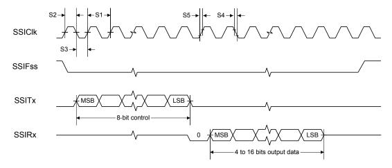
Figure 21-20. Master Mode SSI Timing for SPI Frame Format (FRF=00), with SPH=1
