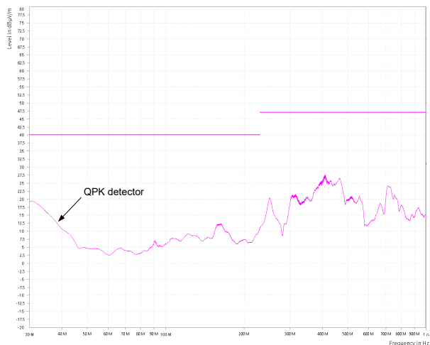
9-9. CISPR 32 Class B Radiated Emissions: Vertical Polarization
