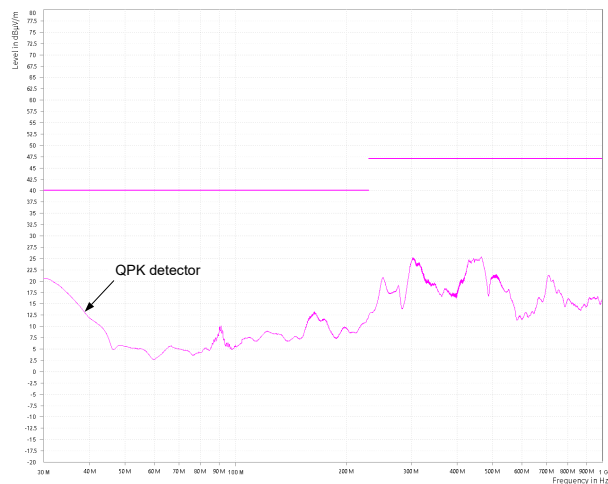
9-8. CISPR 32 Class B Radiated Emissions: Horizontal Polarization
