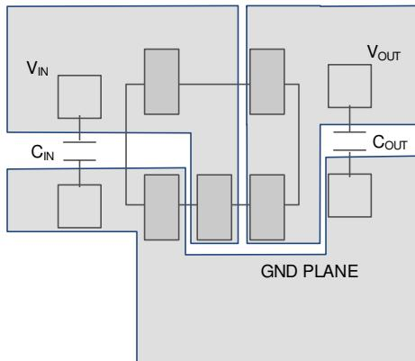
图 8-11. Layout Example for the DBV Package
