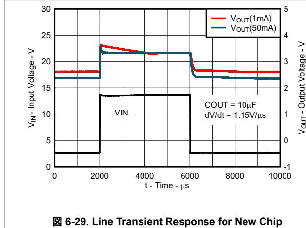
Figure 6-29. Line Transient Response for New Chip
