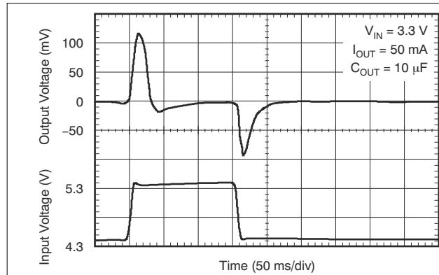
Figure 6-25. Line Transient Response for Legacy Chip
