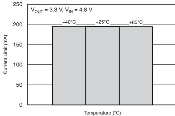
图 6-17. Current Limit vs Junction Temperature for Legacy Chip
