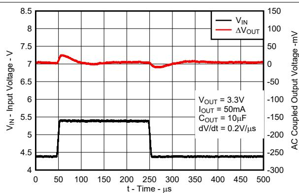
Figure 6-26. Line Transient Response for New Chip
