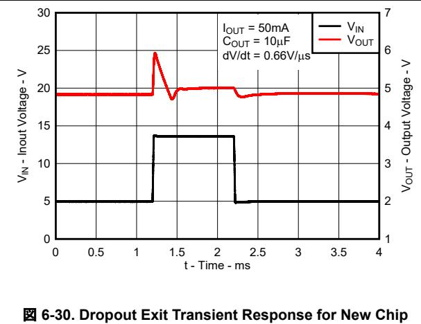
Figure 6-30. Dropout Exit Transient Response for New Chip
