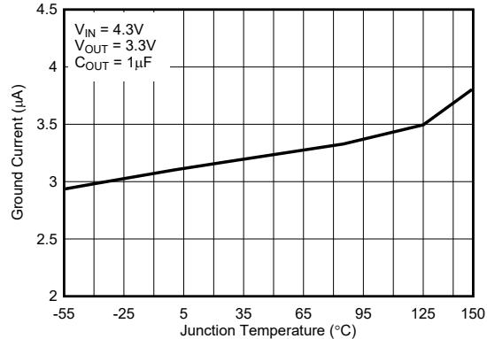
图 6-12. Ground Current vs Junction Temperature for New Chip
