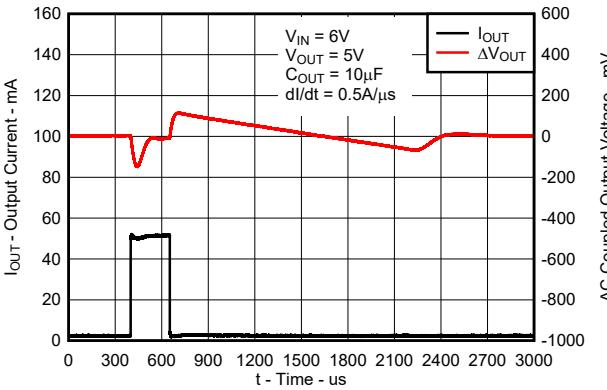
Figure 6-28. Load Transient Response for New Chip
