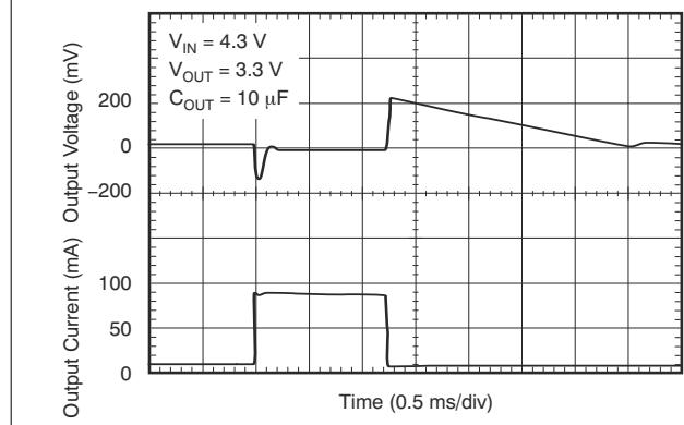
Figure 6-27. Load Transient Response for Legacy Chip
