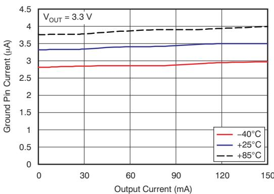
图 6-15. Ground Pin Current vs Load Current for Legacy Chip
