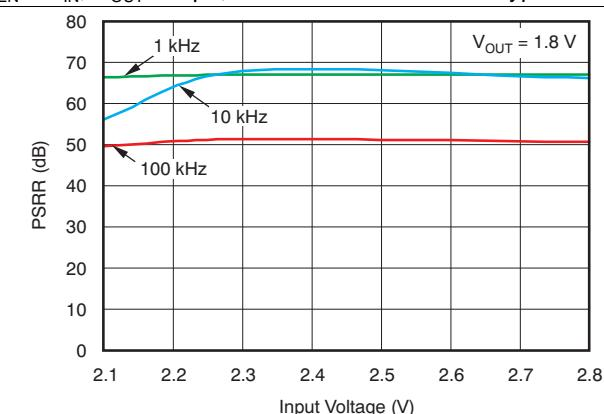
**Figure 13. Power-Supply Ripple Rejection vs Input Voltage**
