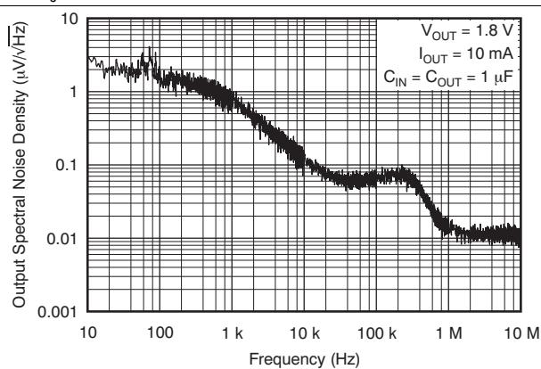
**Figure 14. Output Spectral Noise Density vs Frequency**
