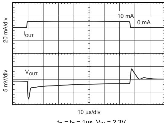
图 5-17. Load Transient Response
