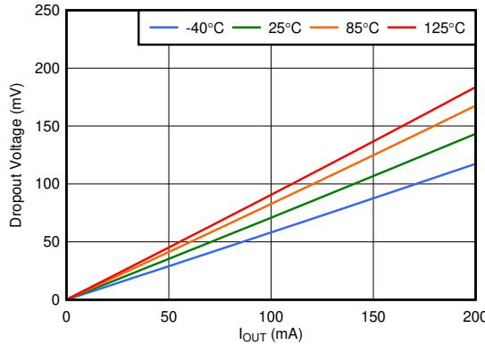
图 5-11. TLV70028-Q1 Dropout Voltage vs Output Current
