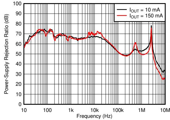
图 5-12. TLV70028-Q1 Power-Supply Rejection Ratio vs Frequency
