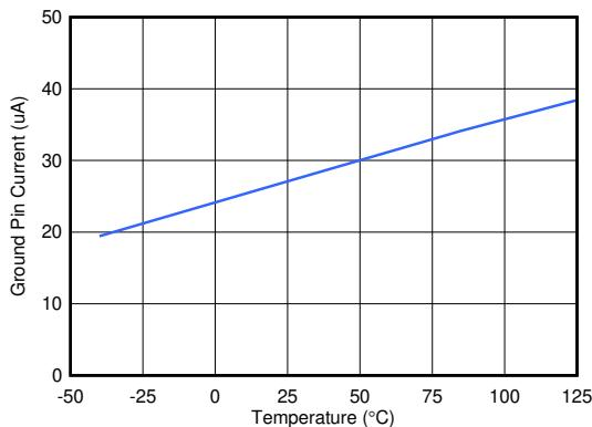
图 5-8. TLV70028-Q1 Ground Pin Current vs Temperature
