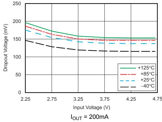
图 5-10. TLV70048-Q1 Dropout Voltage vs Input Voltage
