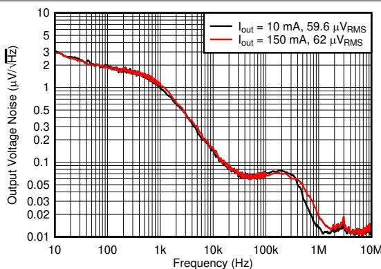
图 5-15. TLV70028-Q1 Output Spectral Noise Density vs Frequency
