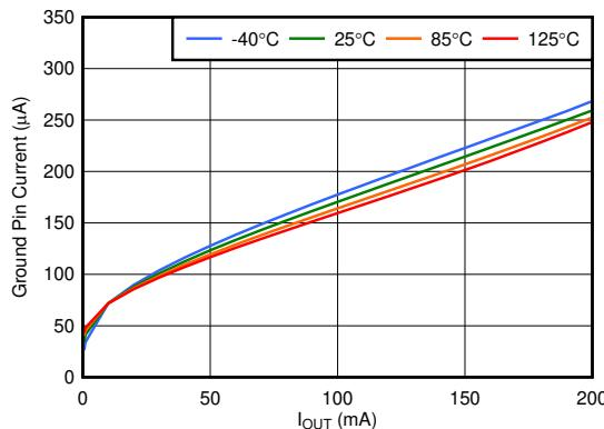
图 5-7. TLV70028-Q1 Ground Pin Current vs Output Current
