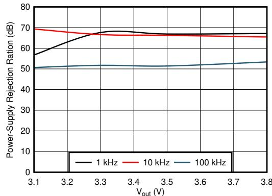
图 5-13. TLV70028-Q1 Power-Supply Rejection Ratio vs Output Voltage
