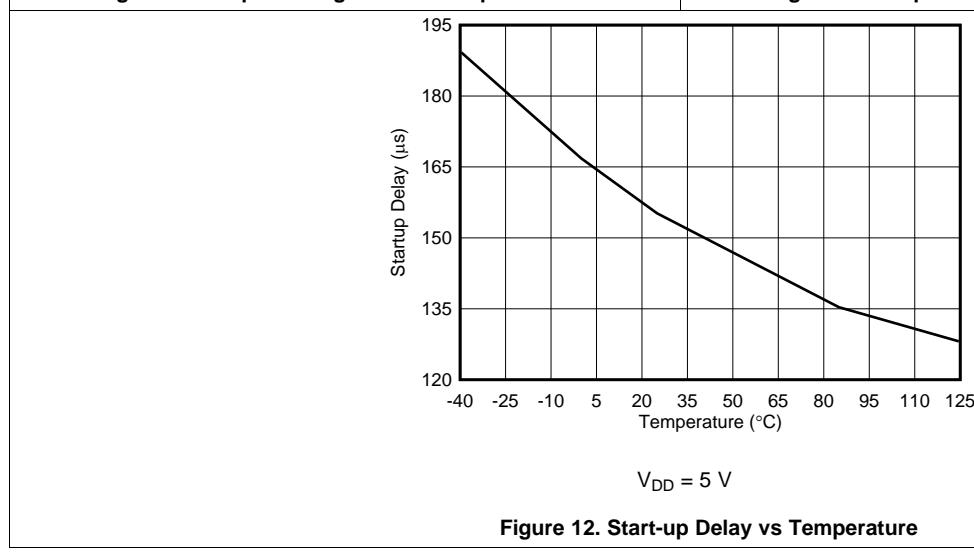
**Figure 12. Start-up Delay vs Temperature**
