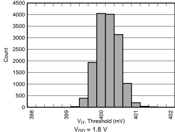
Figure 7. SENSE Negative Input Threshold Voltage ( $V_{IT^-}$ ) Distribution
