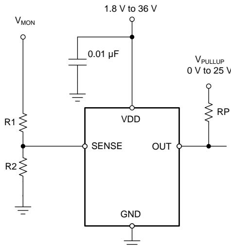
NOTE: The input can monitor a voltage higher than  $V_{DD}$  (maximum) with the use of an external resistor divider network.
