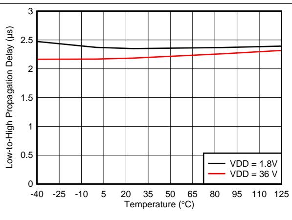
**Figure 9. Propagation Delay vs Temperature
