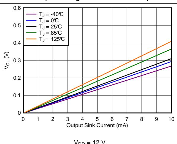
**Figure 11. Output Voltage Low vs Output Sink Current**
