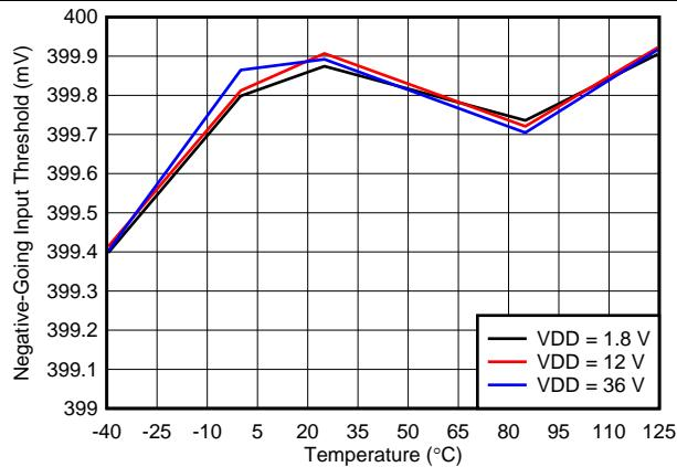
Figure 5. SENSE Negative Input Threshold Voltage ( $V_{IT^-}$ ) vs Temperature
