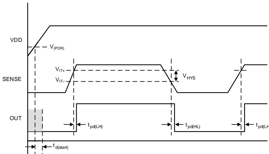
**Figure 1. Timing Diagram**
