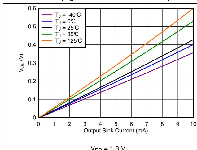
**Figure 10. Output Voltage Low vs Output Sink Current**
