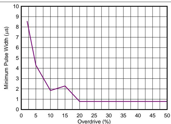
$V_{DD} = 24\text{ V}$ , minimum pulse duration required to trigger output high-to-low transition, SENSE = negative spike below  $V_{IT^-}$
