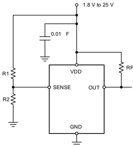
**Figure 13. Monitoring the Same Voltage as  $V_{DD}$**
